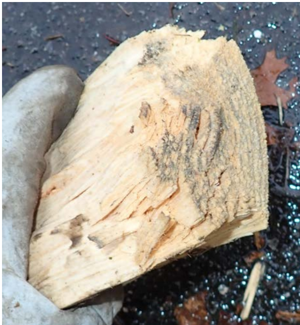
Photo 9: Tree limb damage consistent with propeller strike
