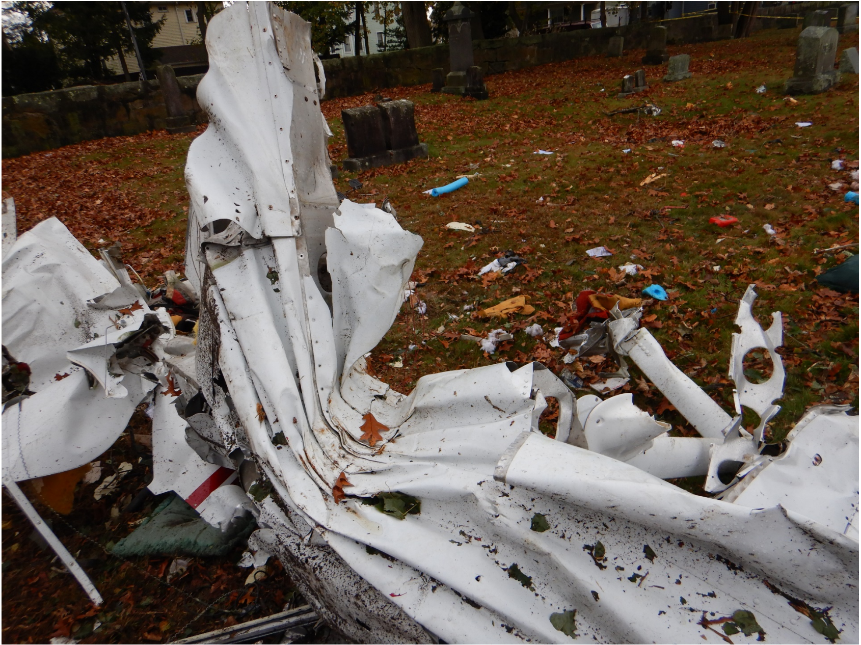
Photo 7 – Right Wing Damage
