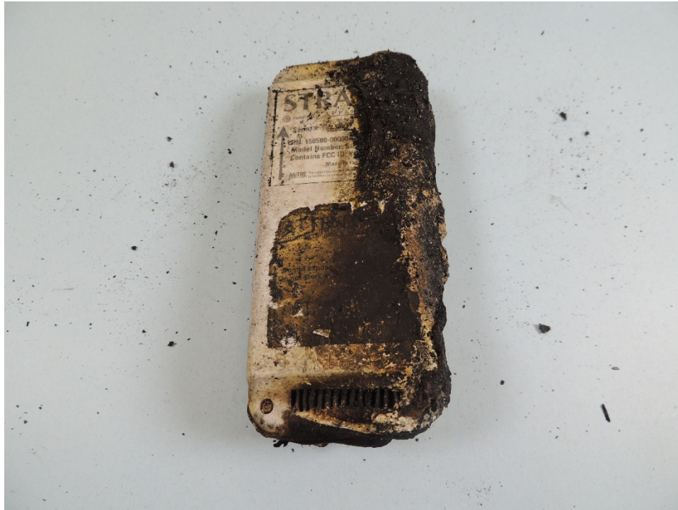
Figure 1. Exterior Damage to Appareo Stratus 2S.
