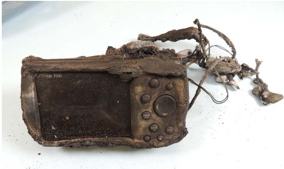
Figure 2. Exterior Damage to Garmin GPSMAP 396.
