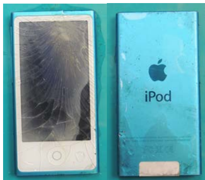
Figure 7. Damaged Apple iPod Nano.
