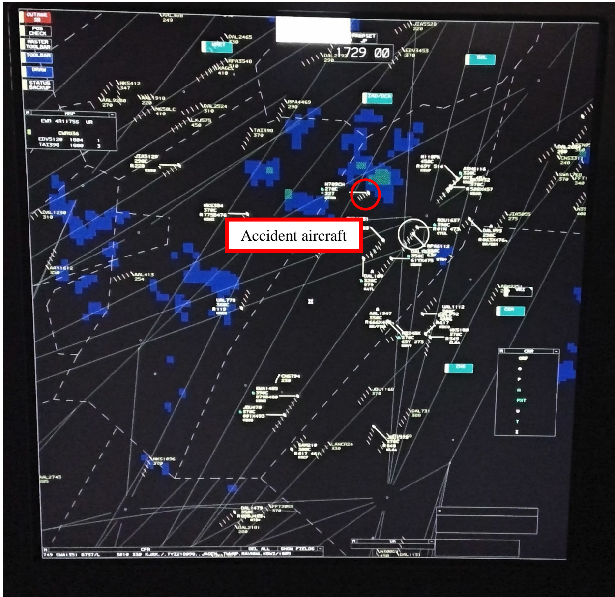
Figure 31 – Screenshot of the ZDC air traffic controller’s radar display at 1329 EDT with WARP derived weather displayed
