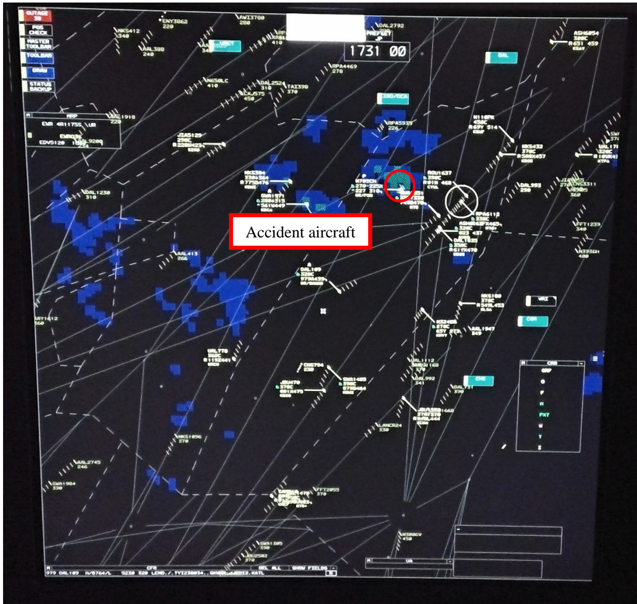
Figure 32 – Screenshot of the ZDC air traffic controller’s radar display at 1331 EDT with WARP derived weather displayed
