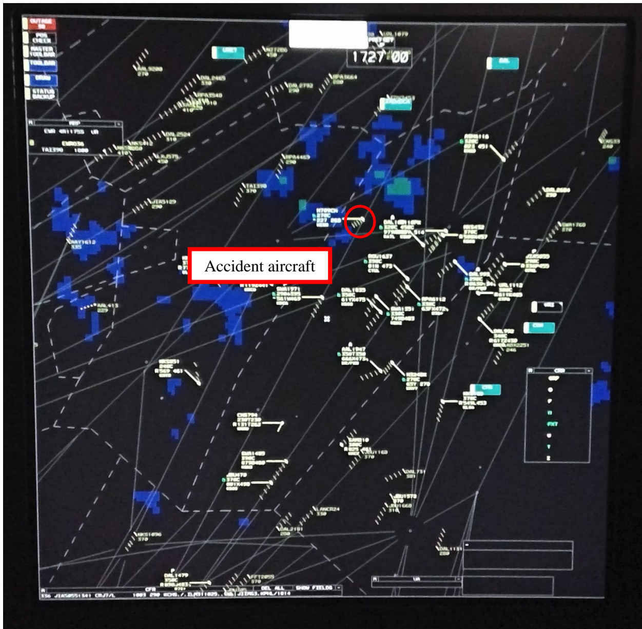
Figure 30 – Screenshot of the ZDC air traffic controller’s radar display at 1327 EDT with WARP derived weather displayed
