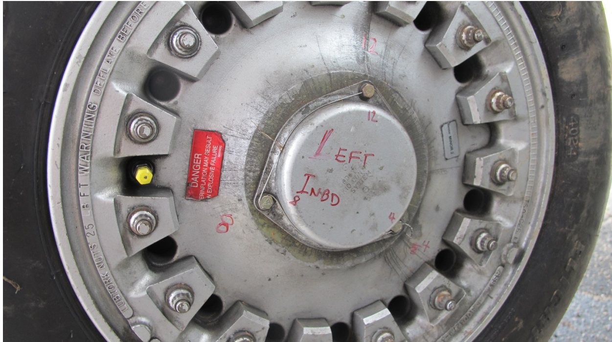
Figure 9 - Left inboard wheel/tire assembly prior to hub removal
