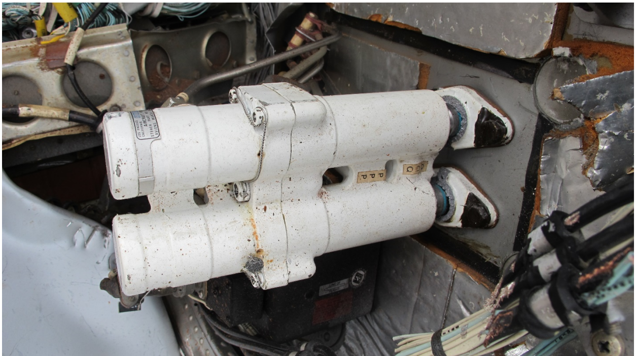
Figure 37 - Normal/Emergency Brake Selector Valve with fractures at the pressure bulkhead
