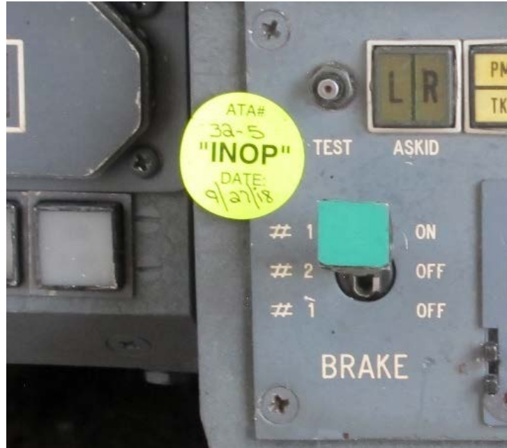
Figure 7 – Brake switch showing “INOP” sticker closeup
