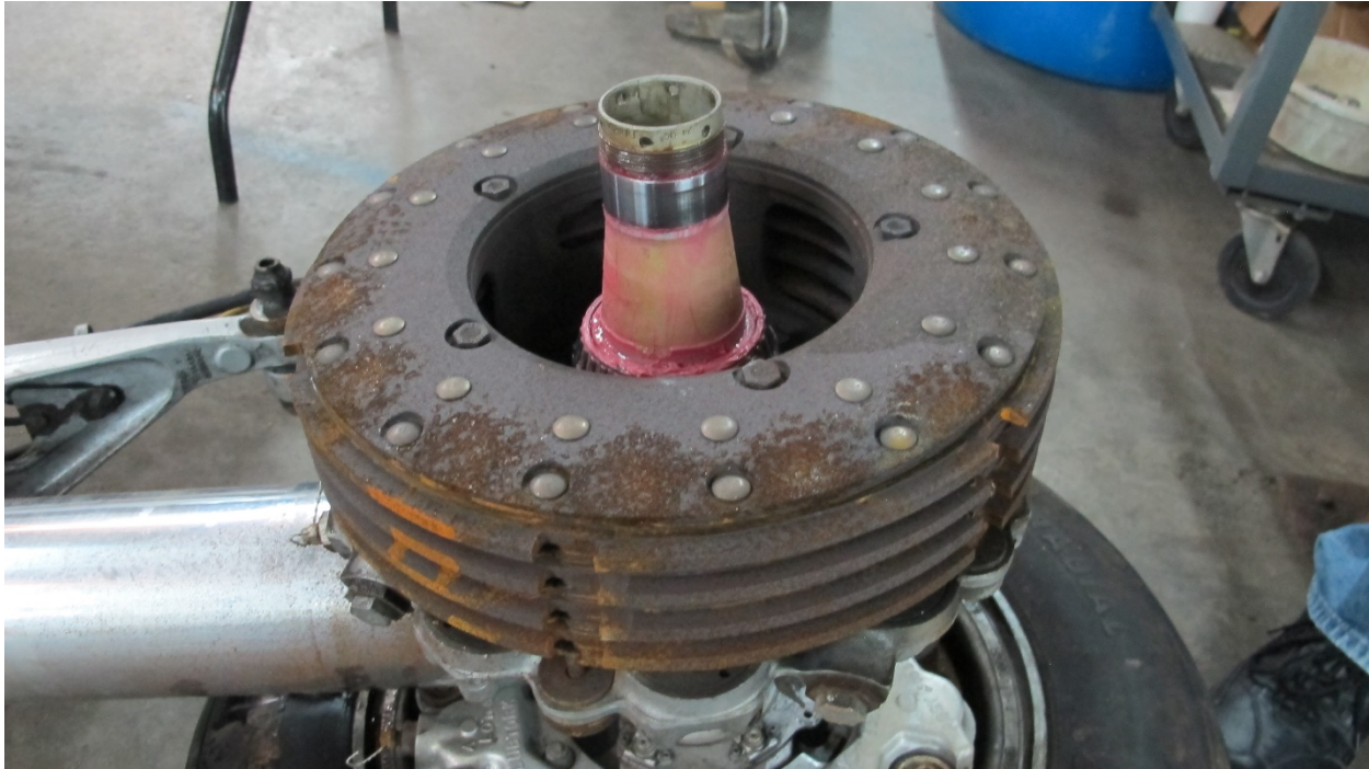
Figure 33 - RH Inboard brake assembly, wheel removed
