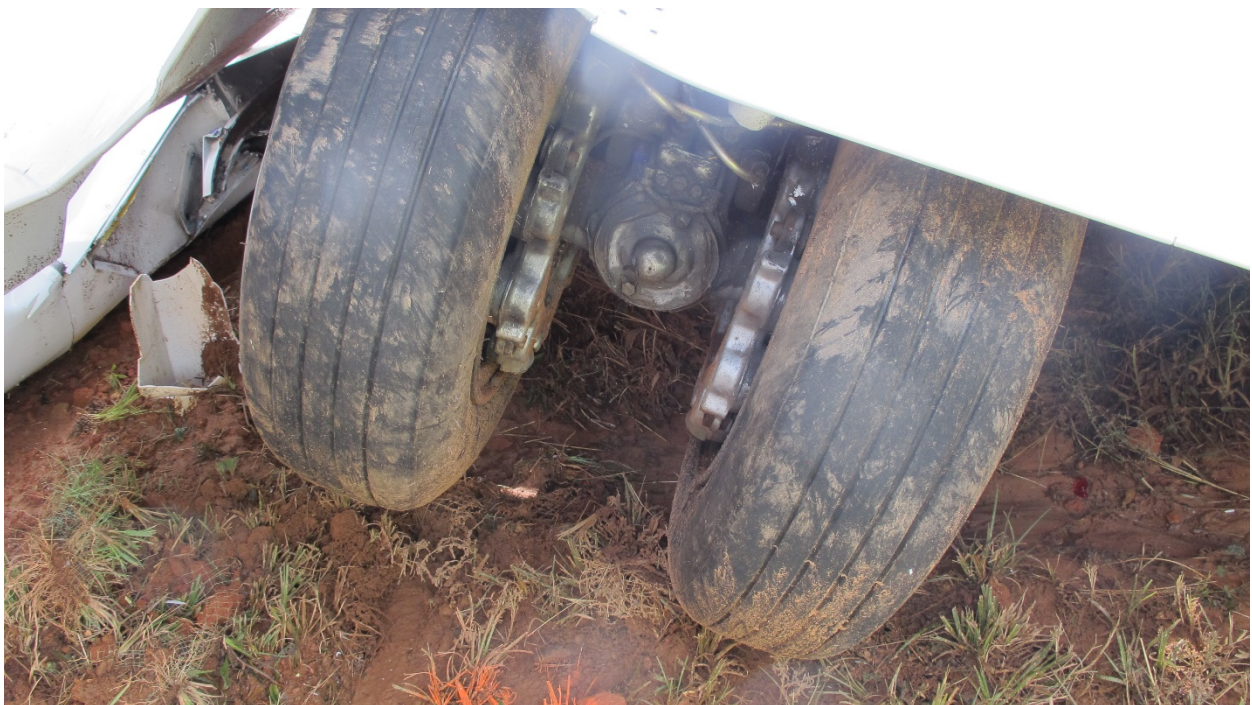
Figure 31 - RH Main gear as found
