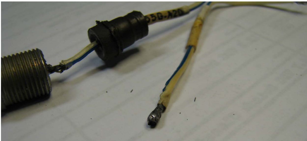
Figure 18 - Broken wire to pin on wheel speed transducer connector
