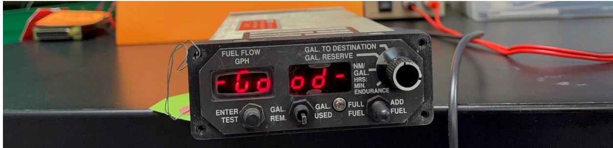
Figure 3. The Shadin Miniflo-L™ self test upon power up.
