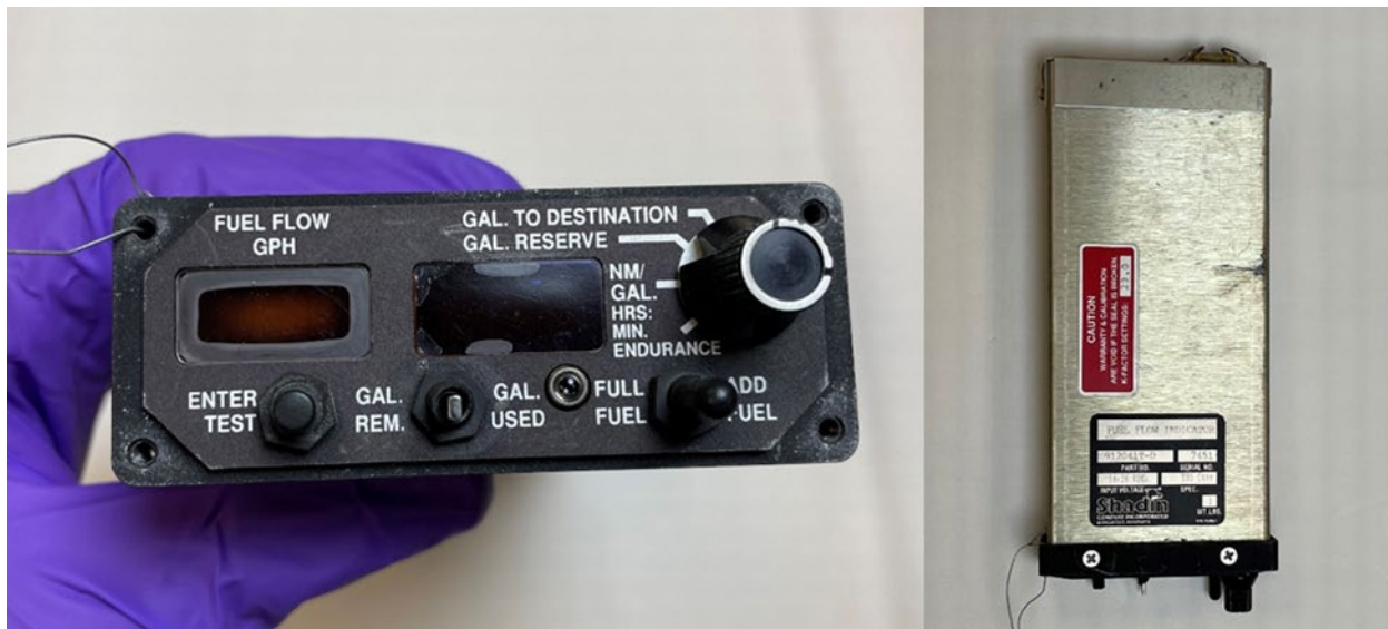
Figure 2. Front and top view of Shadin Miniflo-L™, as received.
