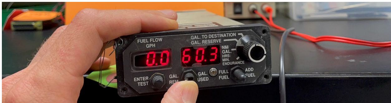
Figure 5. The Shadin Miniflo-L™ indicating the amount of fuel remaining.
