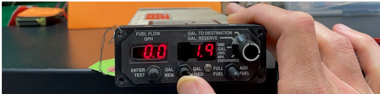
Figure 4. The Shadin Miniflo-L™ indicating the amount of fuel used.
