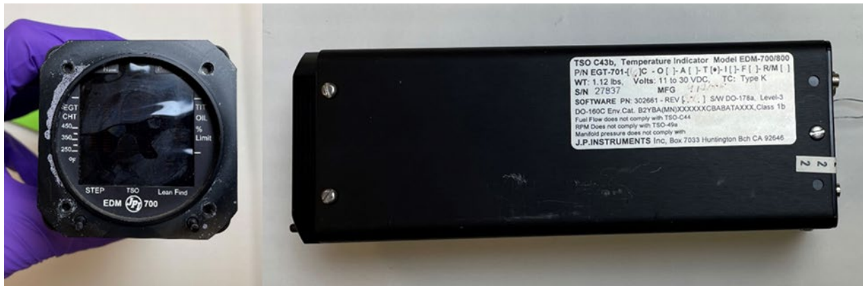
Figure 1. Front and side view of EDM-700, as received.
