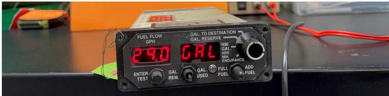
Figure 6. The Shadin Miniflo-L™ indicating the K-factor setting (left) and units of measure (right).
