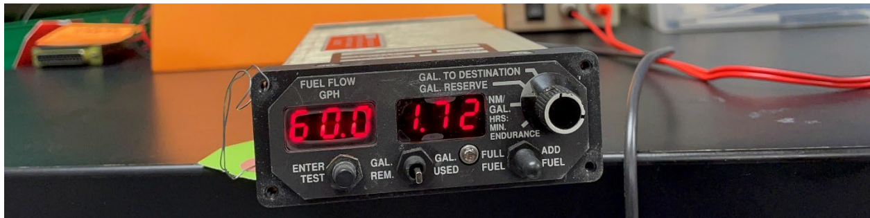
Figure 9. The Shadin Miniflo-L™ indicating the software version.
