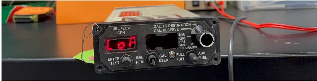
Figure 7. The Shadin Miniflo-L™ indicating no Loran/GPS signal.
