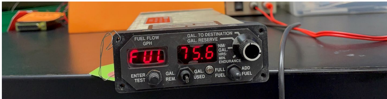
Figure 8. The Shadin Miniflo-L™ indicating the maximum usable fuel.
