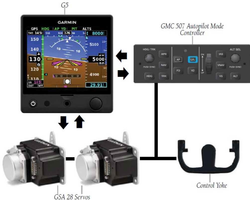
Figure 1. Garmin 500 Auto Flight Control System general schematic (courtesy of Garmin, taken from the G5 Electronic Flight Instrument Pilot's Guide for Certified Aircraft ).
