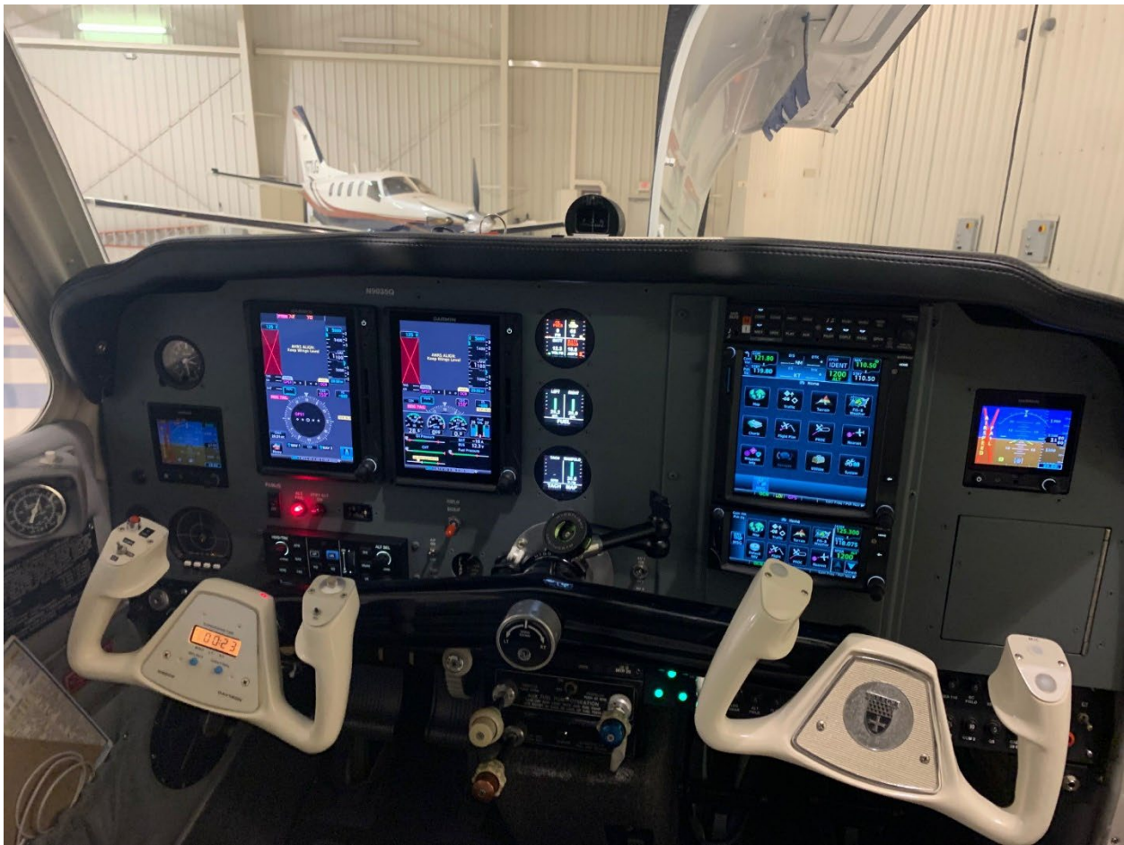
Figure 2. The airplane's flight deck and autopilot installation.
