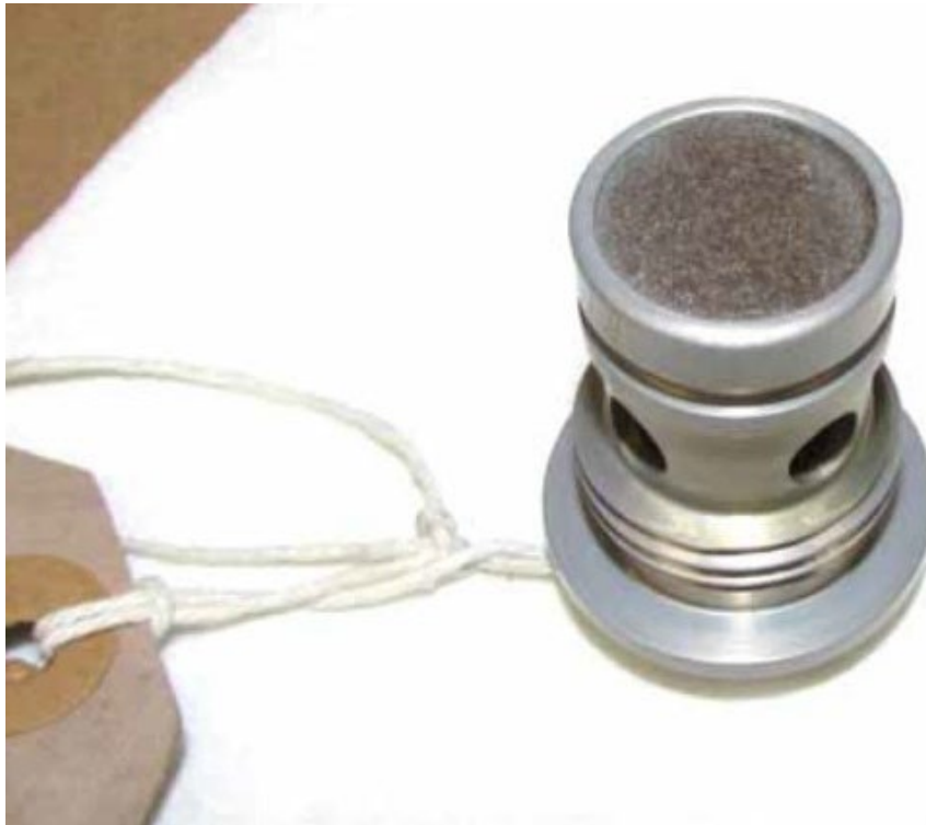
Photo 34 – Fuel Pump Lube Flow Screen – Partially Blocked
