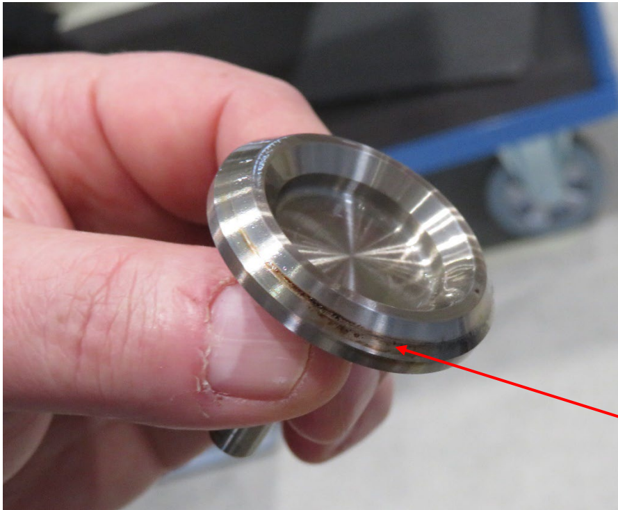
Photo 32 - Fuel Filter Bypass Valve – Conical Valve
