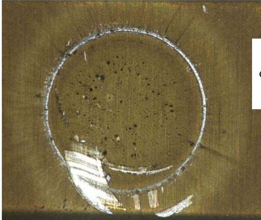
Photo 19 – Flapper Valve ‘Sun Ray’ Contact Marks with Nozzle
