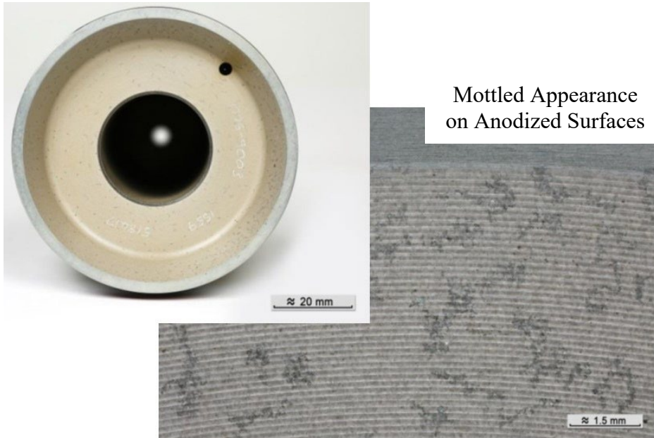
Photo 25 – VSV Actuator Piston Surface Corrosion
