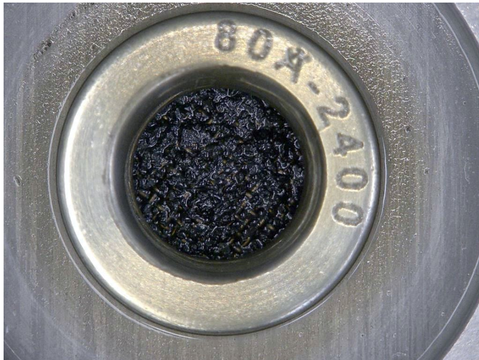
Photo 14 – Torque Motor Supply Port (70 - 80 \mu ) Filter Element (wet)
