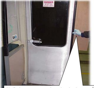
Verify door operator arm is against the door stop and then apply finger pressure to push the door toward the pocket to remove any slack in the mechanism. Set the dial indicator to "0".
