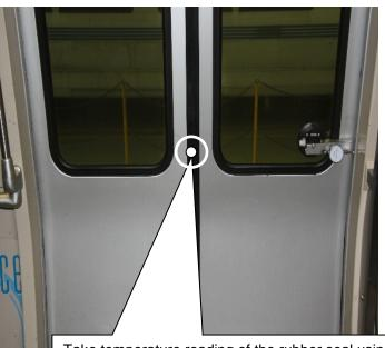
Take temperature reading of the rubber seal using the infrared thermometer, approximately 2 inches away and perpendicular to target.
