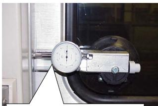
Attach dial indicator to window and position to contact metal trim within 6 inches above the bottom of the window.
