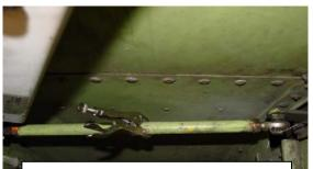
Loosen jam nuts and rotate the linkage rods to center the doors or to increase or decrease the amount of "push"
