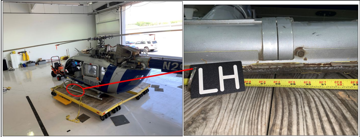
Figure 13: Overview of helicopter skid and dolly related witness marks.
