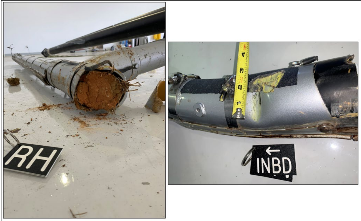
Figure 15: Overview of helicopter skid and dolly related witness marks.
