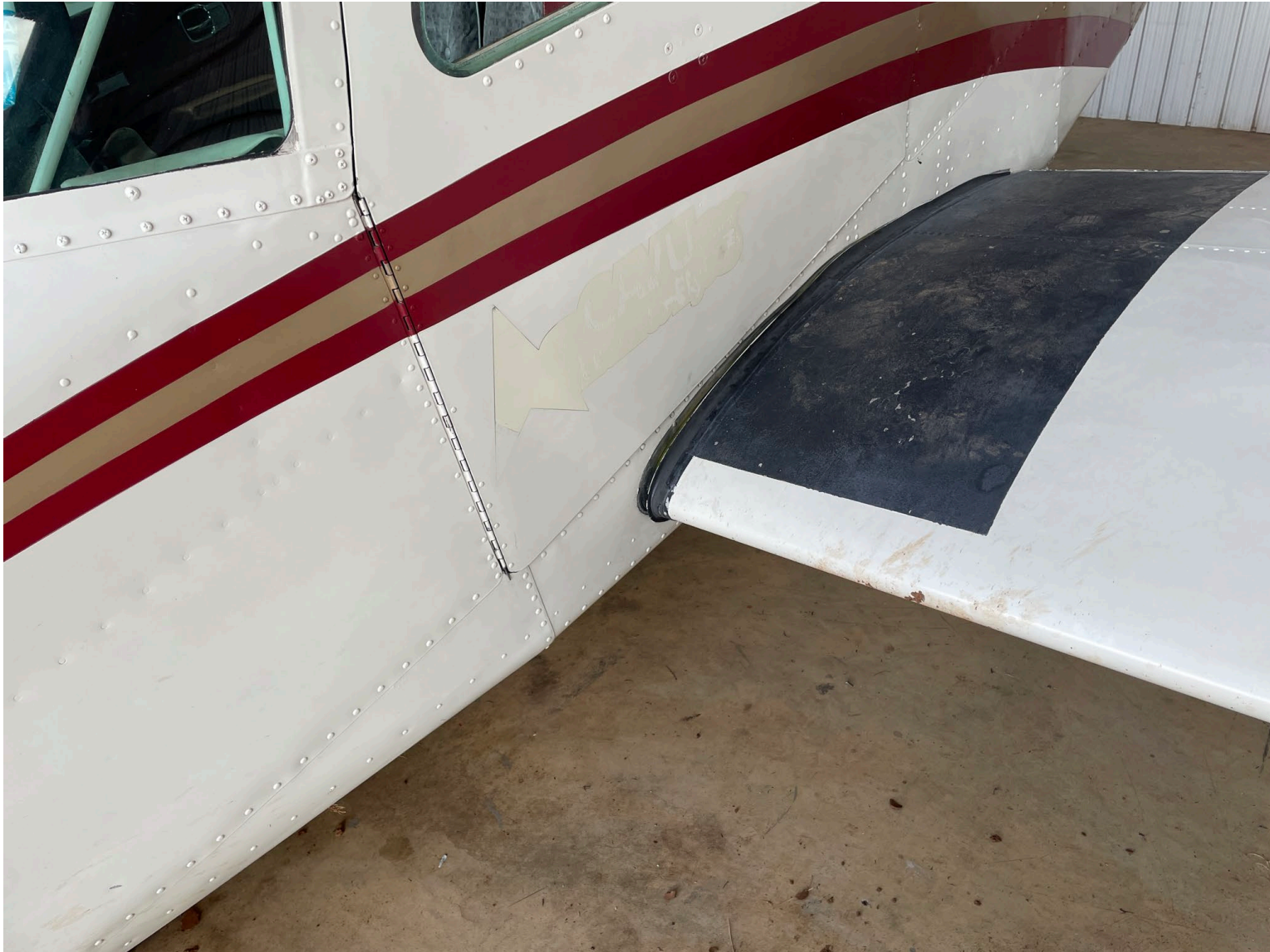
Photograph 3 - Left wing separation (Courtesy of FAA)
