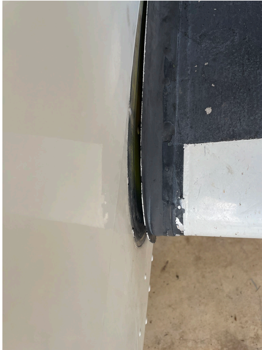
Photograph 4 - Left wing separation (Courtesy of FAA)
