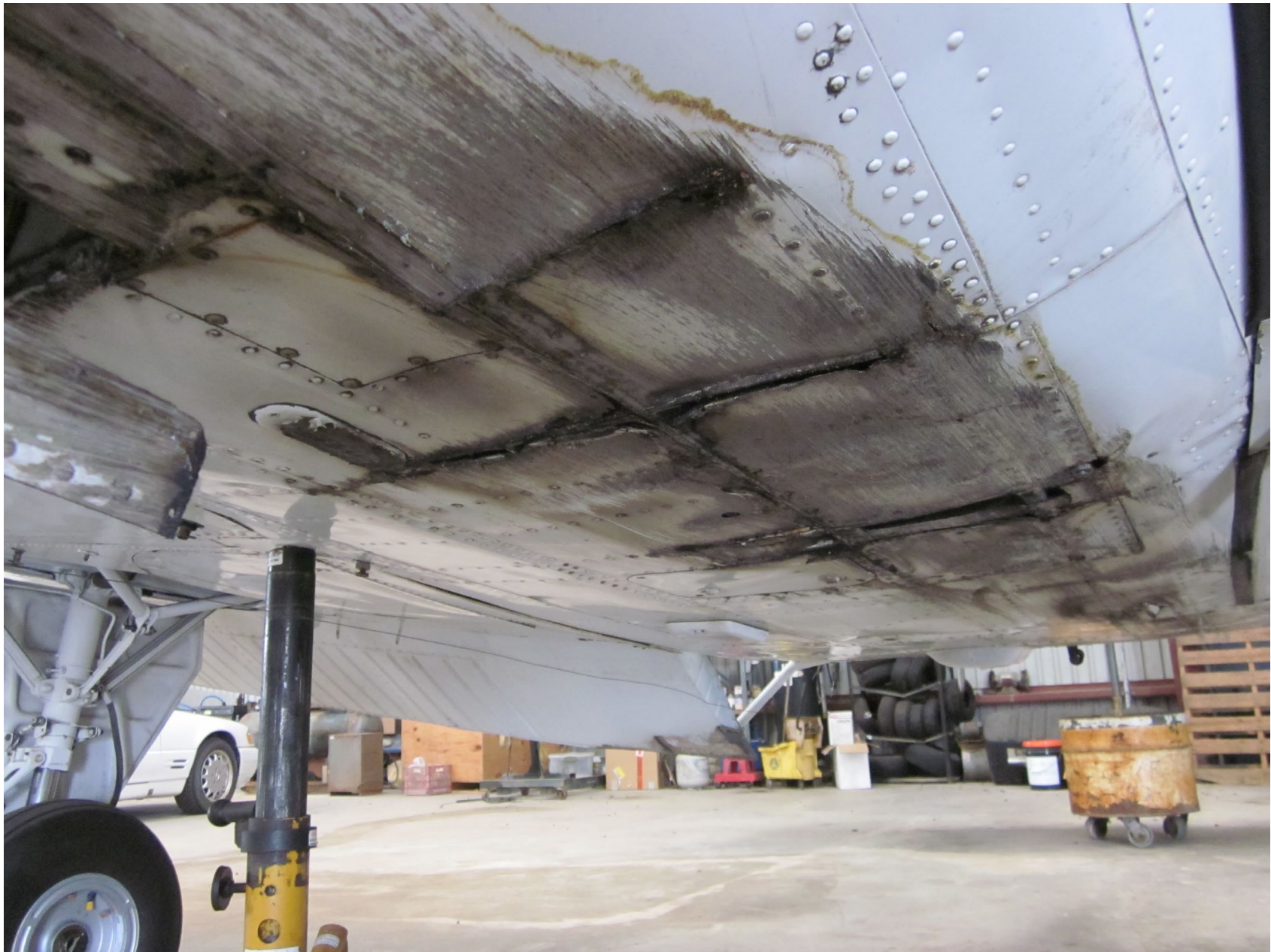
Photo 1 – View of the damaged flap (Courtesy of Federal Aviation Administration) - FAA
