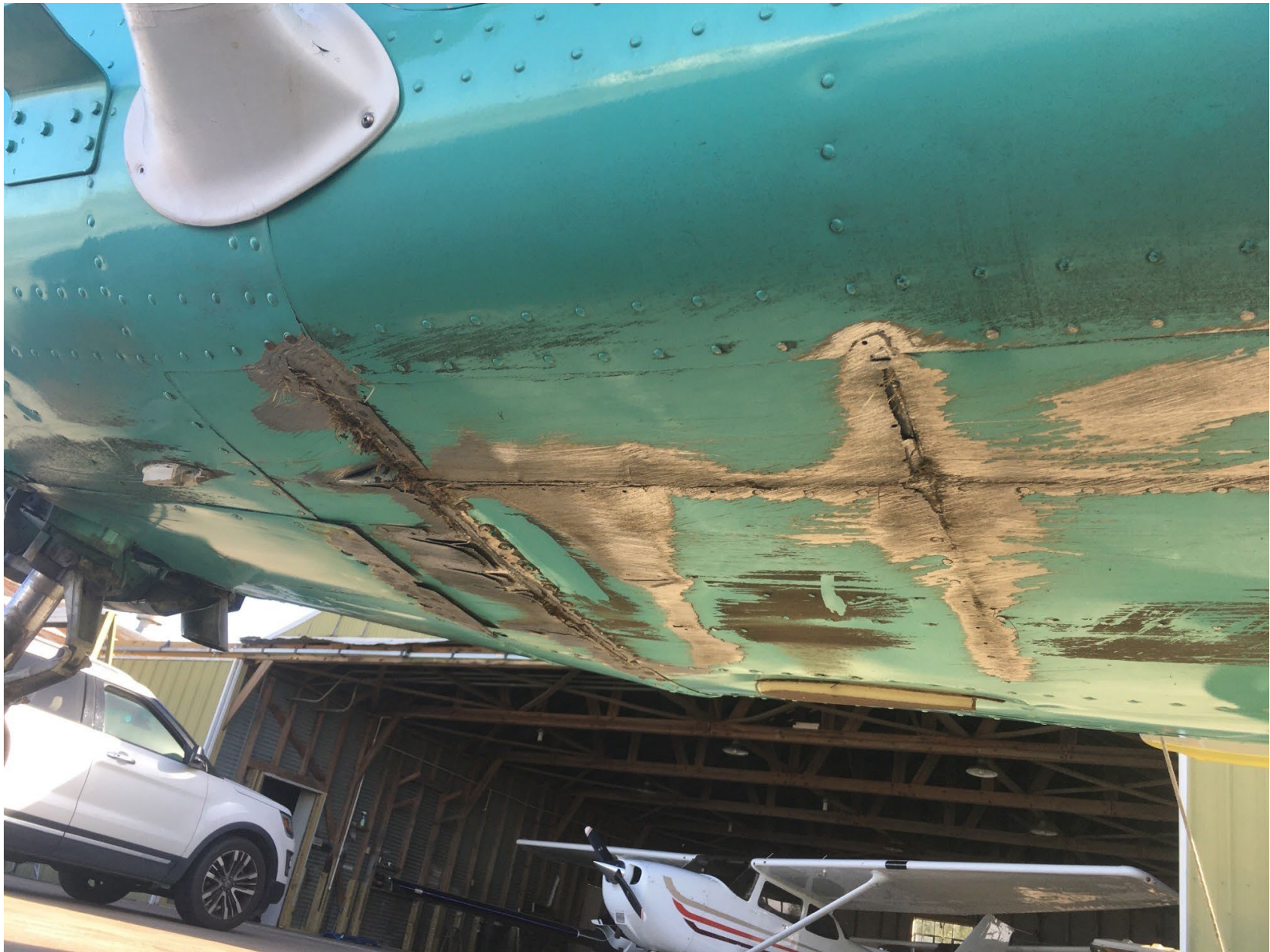
Photo 2 – Structural Damage to Bulkhead (Courtesy of Federal Aviation Administration)
