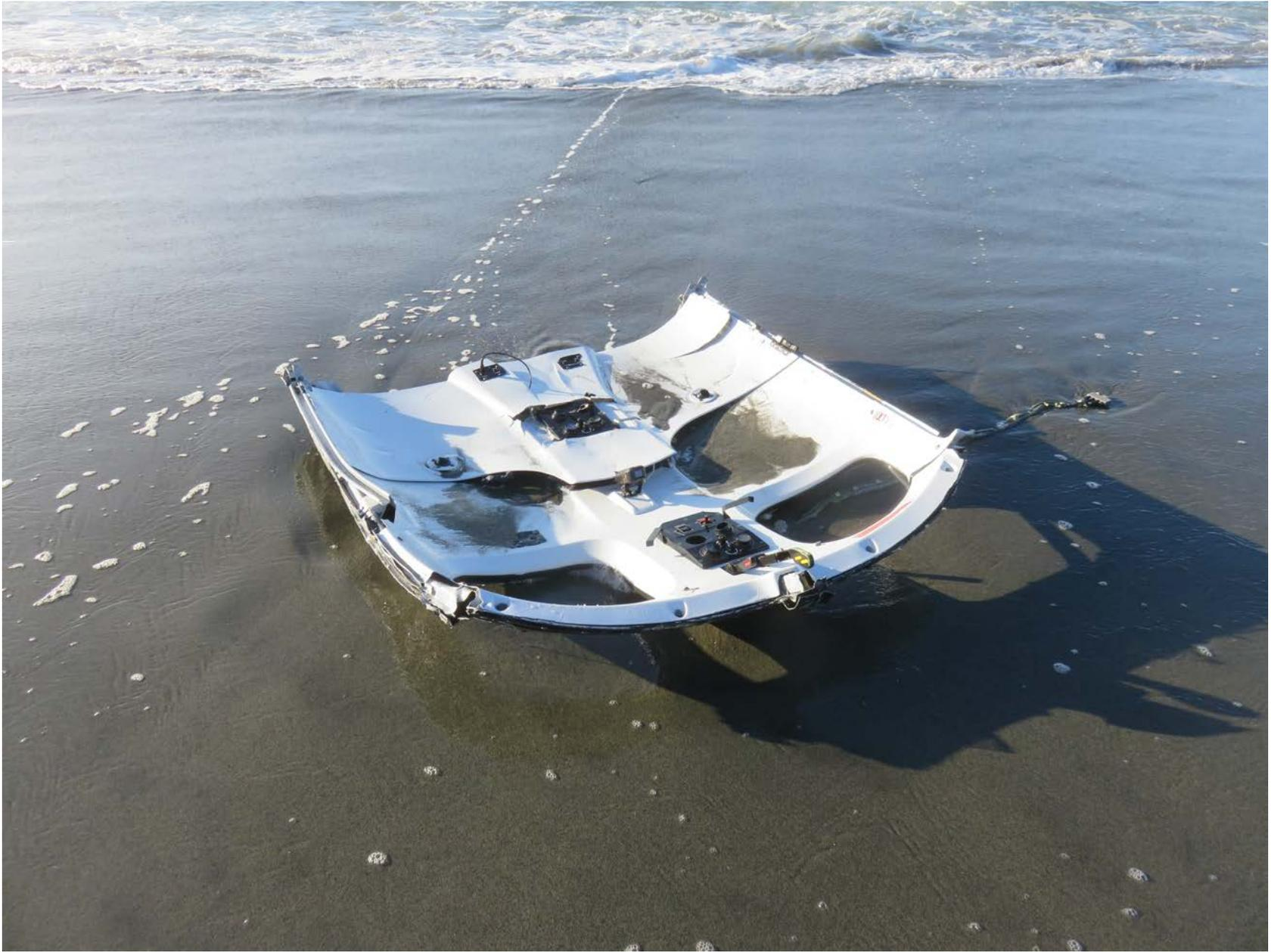
**Photo 6 – Top of cabin structure with Vision 1000**
