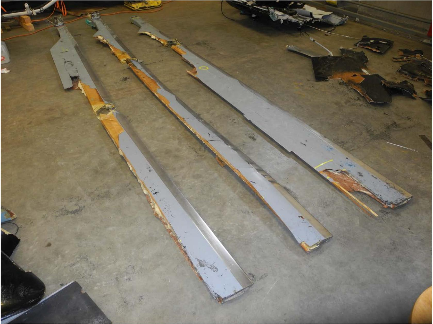
**Photo 9 – Damaged main rotor blades**
