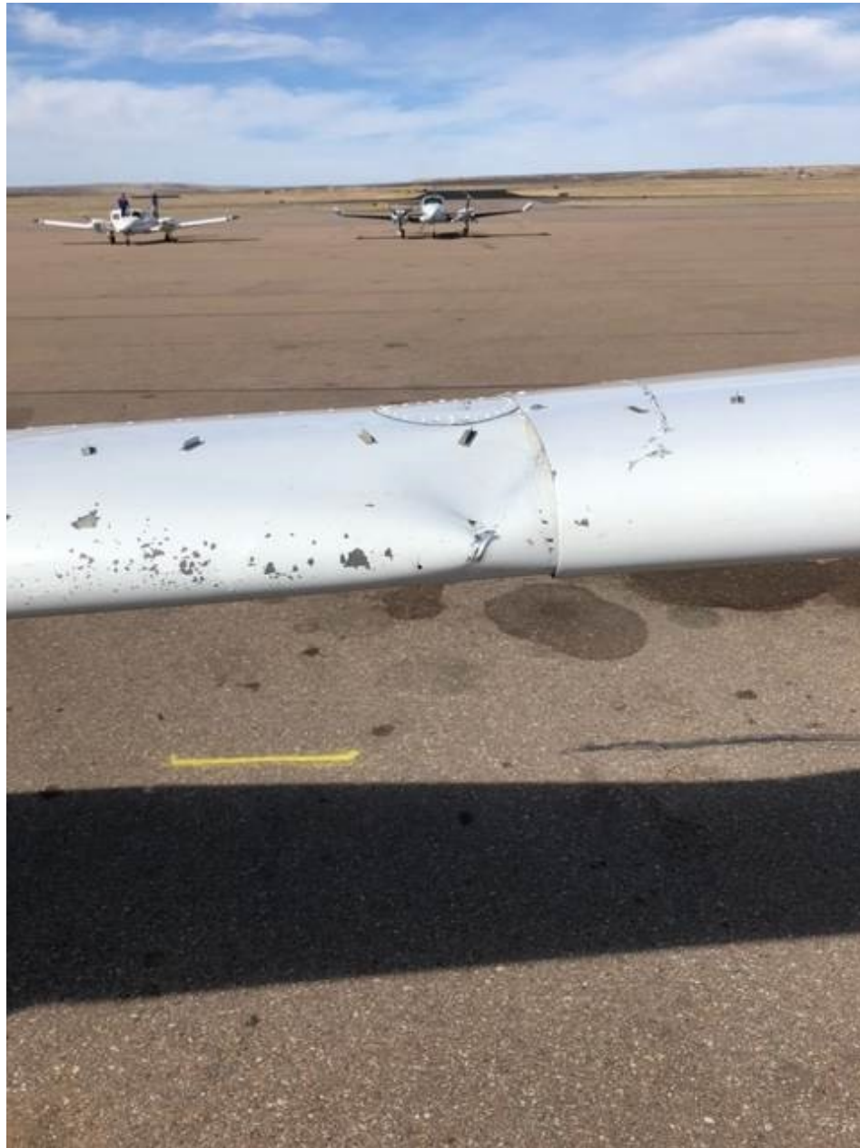
Photo 2 – Left Wing Damage (Courtesy of the owner)
