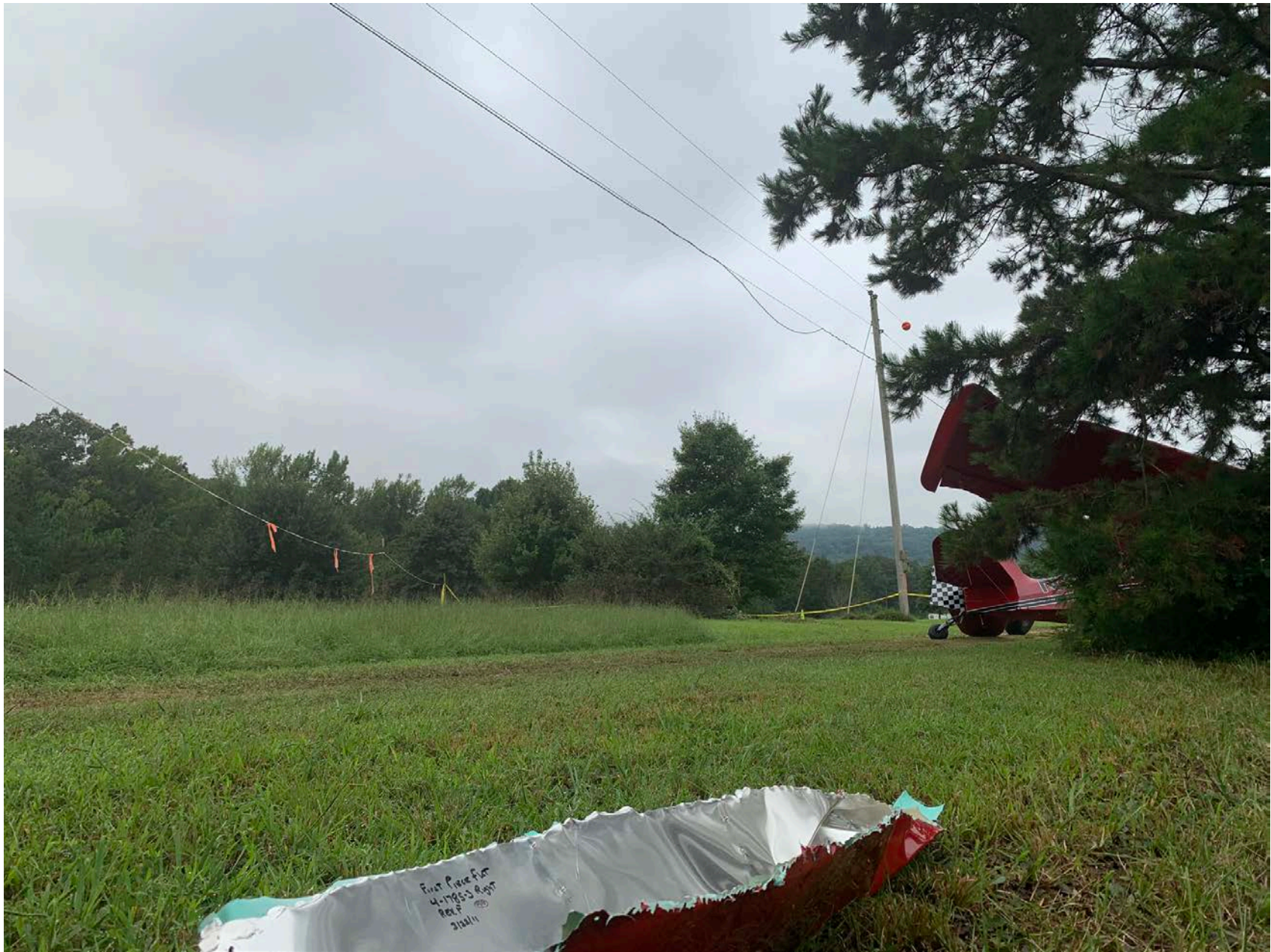
Photo 3 – Power lines and a piece of right wing leading edge
