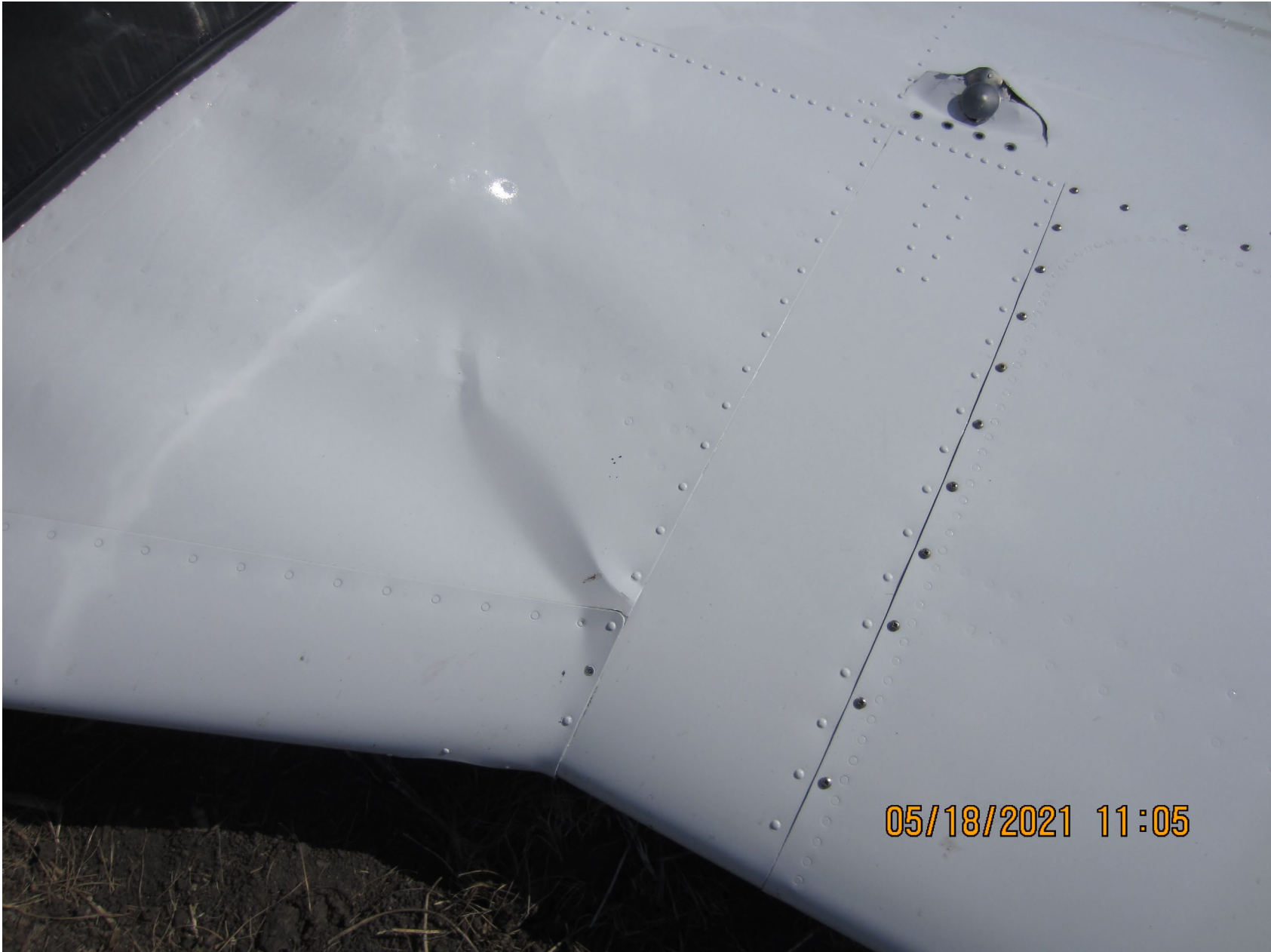
Photo 2 – Left Wing Damage
