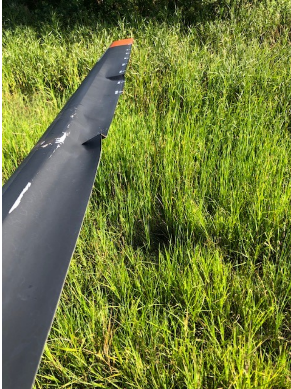
Photo 1 – Main Rotor Blade Damage
