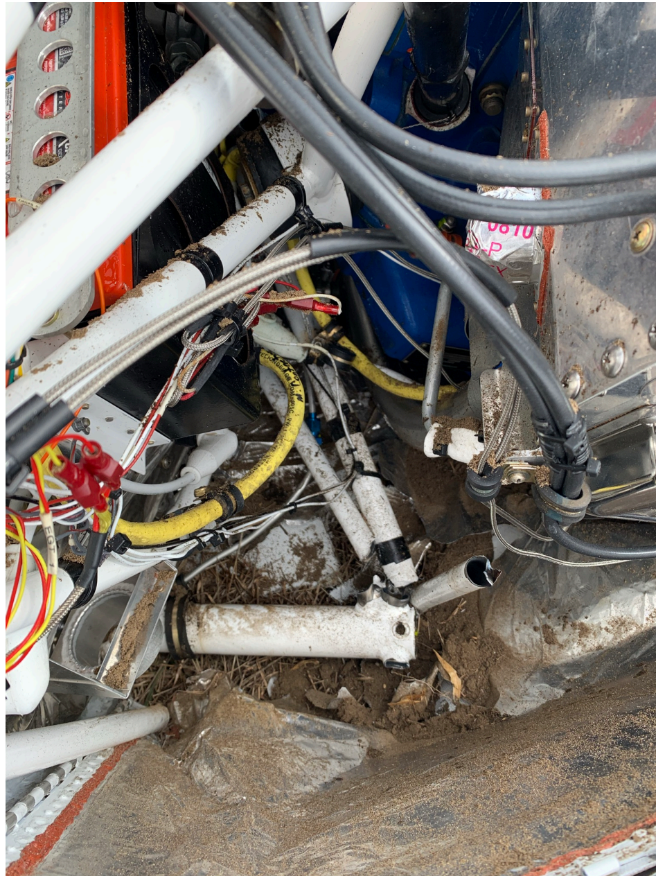
Photo 2 - View of Fractured Engine Mounts and Fuselage Damage (FAA)
