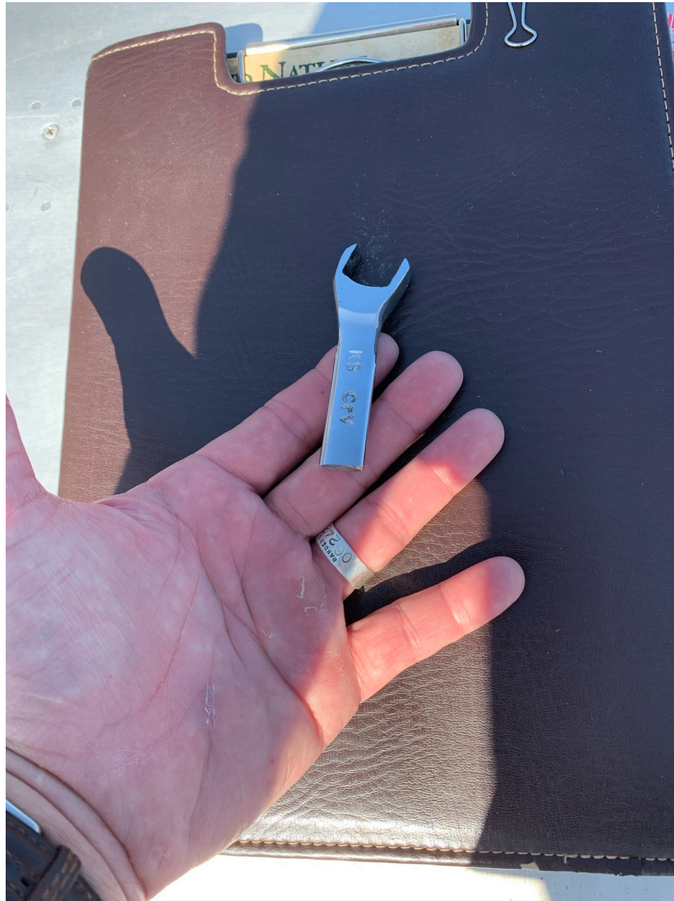
Photo 5 - View of Owner's Modified Spanner Wrench (FAA)
