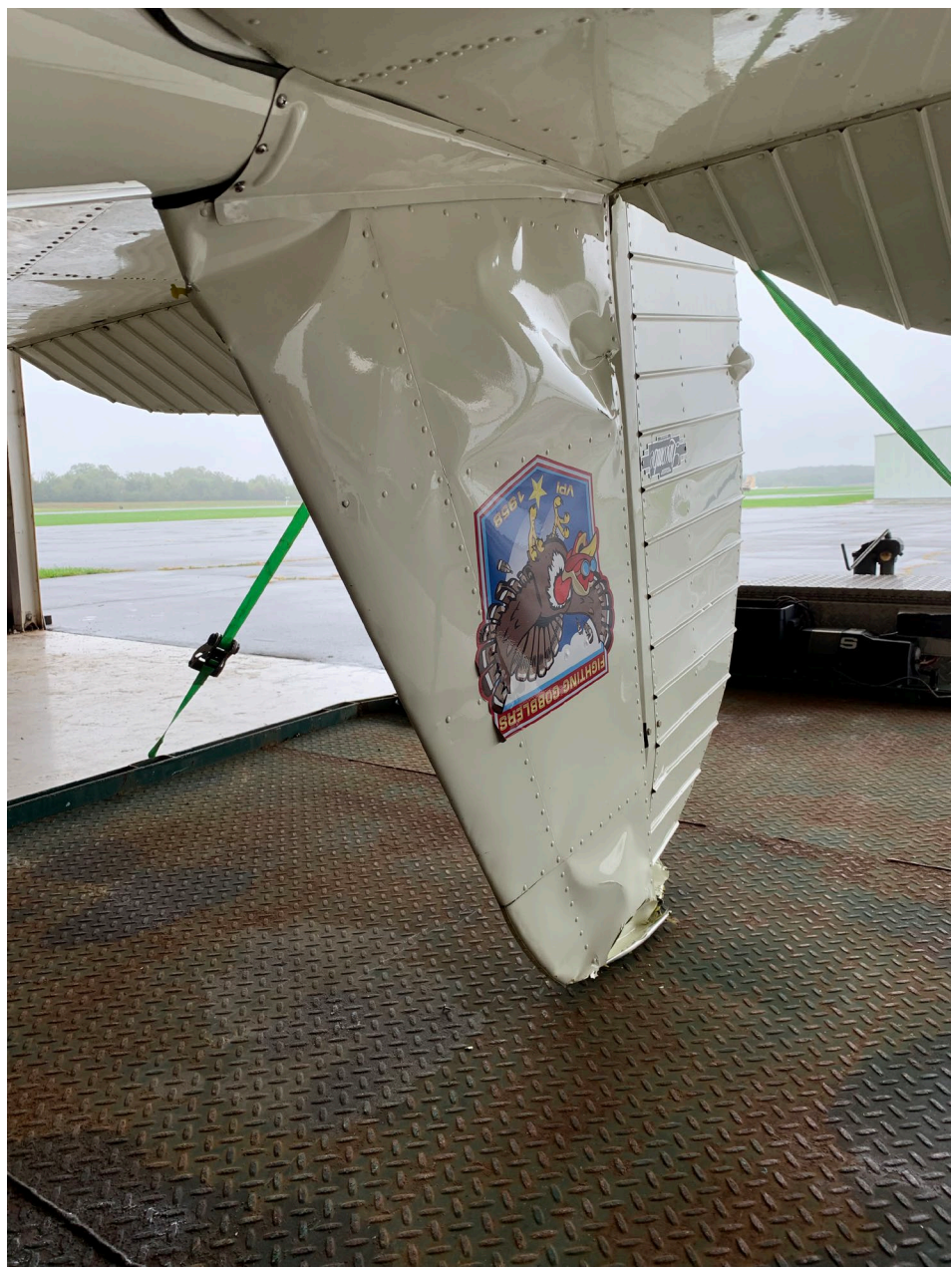
Photo 1 – View of Substantial Damage to Vertical Fin. (FAA)
