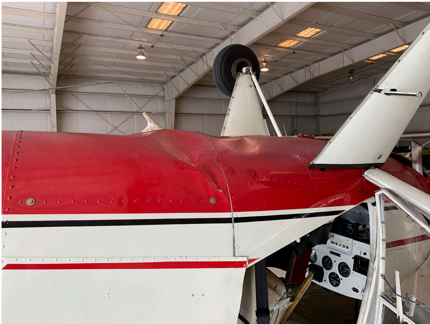
Photo 2 – View of Fuselage Buckling aft of Cockpit (FAA)
