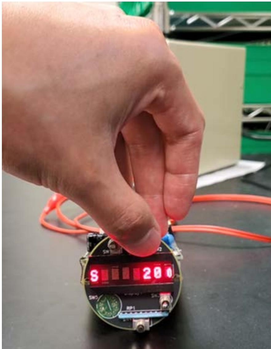
Figure 3: Low Fuel Level setting in device's Entry Mode.
