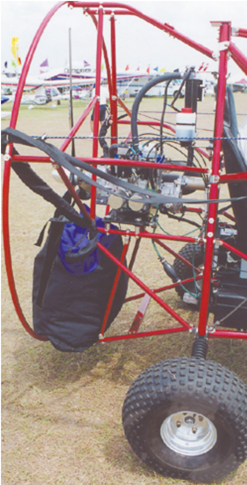
COMPACT PACKAGE – With its canopy stowed, the Destiny 2000 won't require a large trailer to transport it. Of course, you can't taxi it with the canopy in this location.
