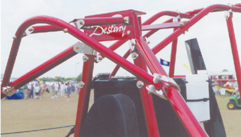
ROLL BAR – Also new for 2000 was this roll bar, which better protects someone in the aft seat. The method of attachment uses standard parts from the Destiny design.
