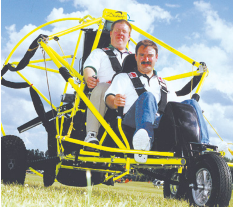
ALL SEATED – Charlie Brown takes the rear seat with Destiny designer and company owner John Rivers in front. Note the dual throttle controls and the standard 5-point pilot and passenger restraints.
