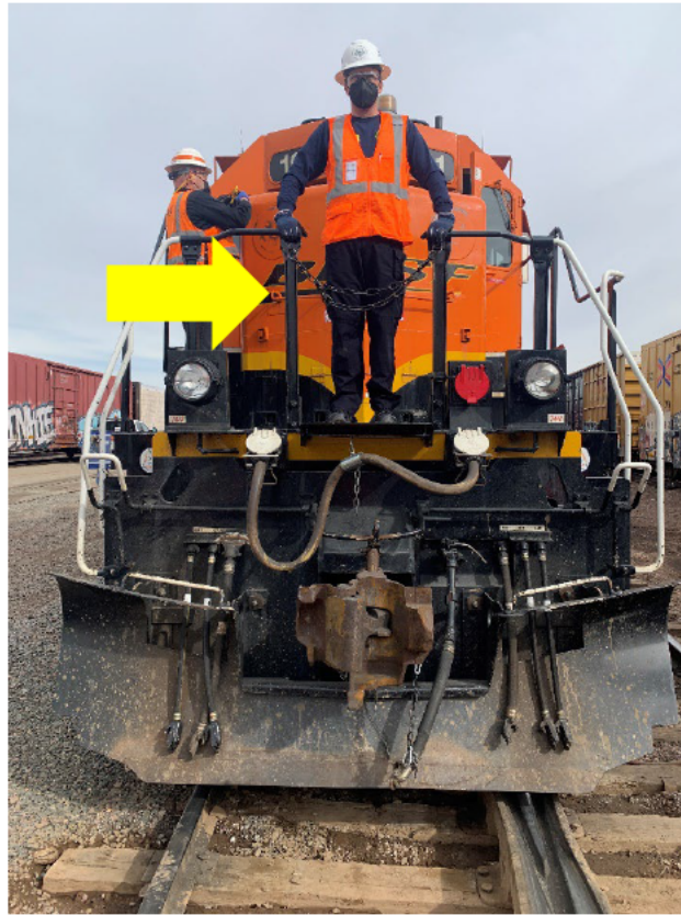
Figure 1: NTSB Investigator standing on the nose platform of the locomotive. The yellow arrow indicates the position of the continuous barrier chain. Source NTSB.
