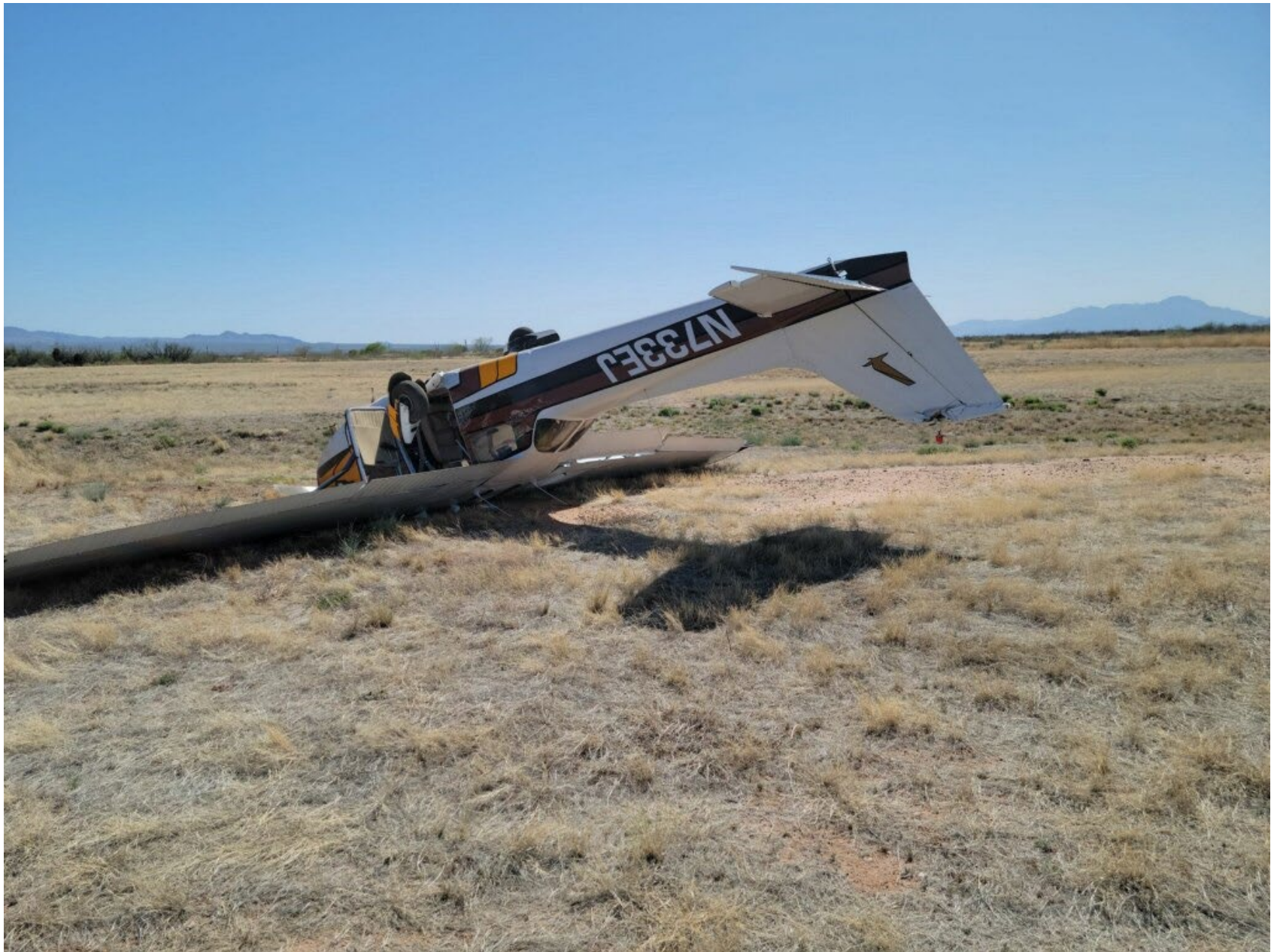
Photo 2 - View of the vertical stabilizer and rudder damage (photo courtesy of the pilot)
