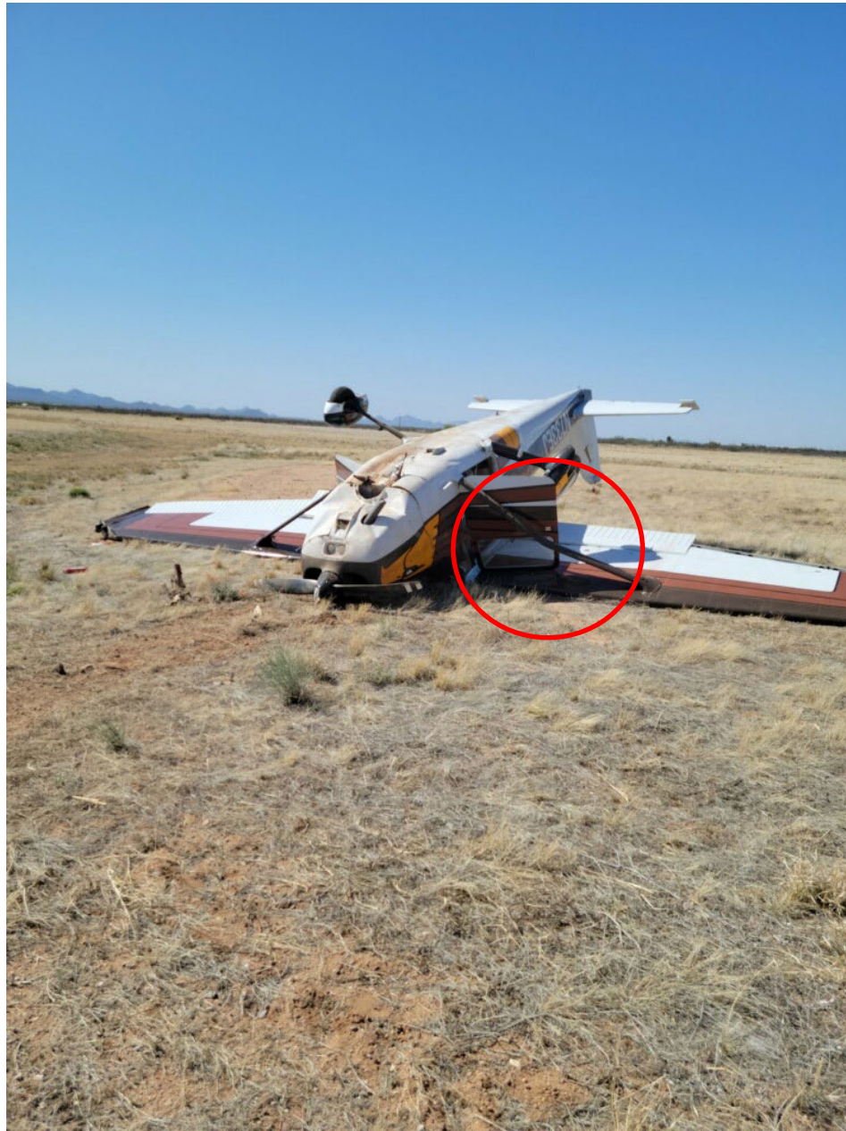
Photo 1 – View of the right-wing lift strut damage (photo courtesy of the pilot)
