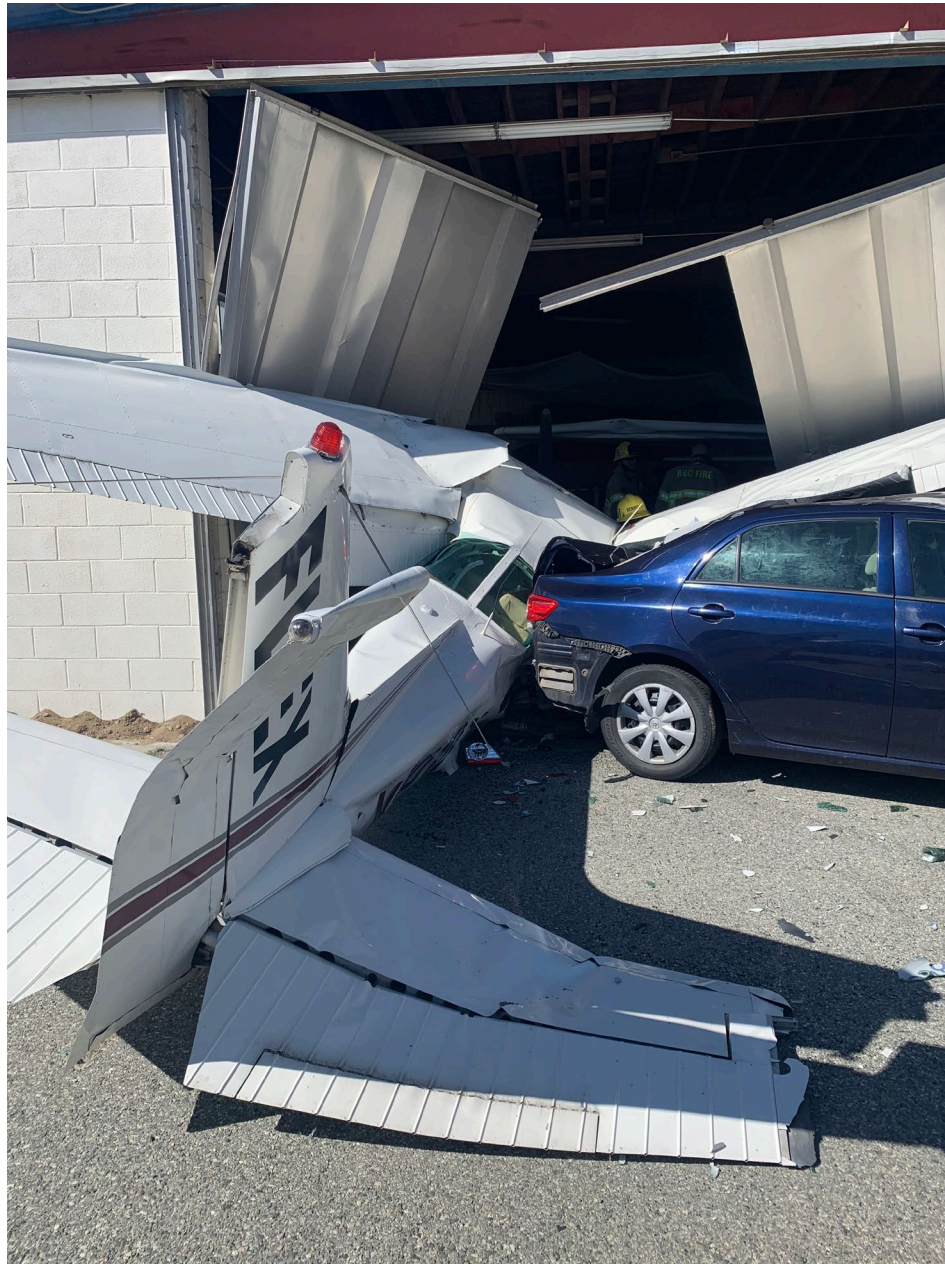
Photo 1 – Rear view of fuselage and wing damage (photo courtesy of local law enforcement)
