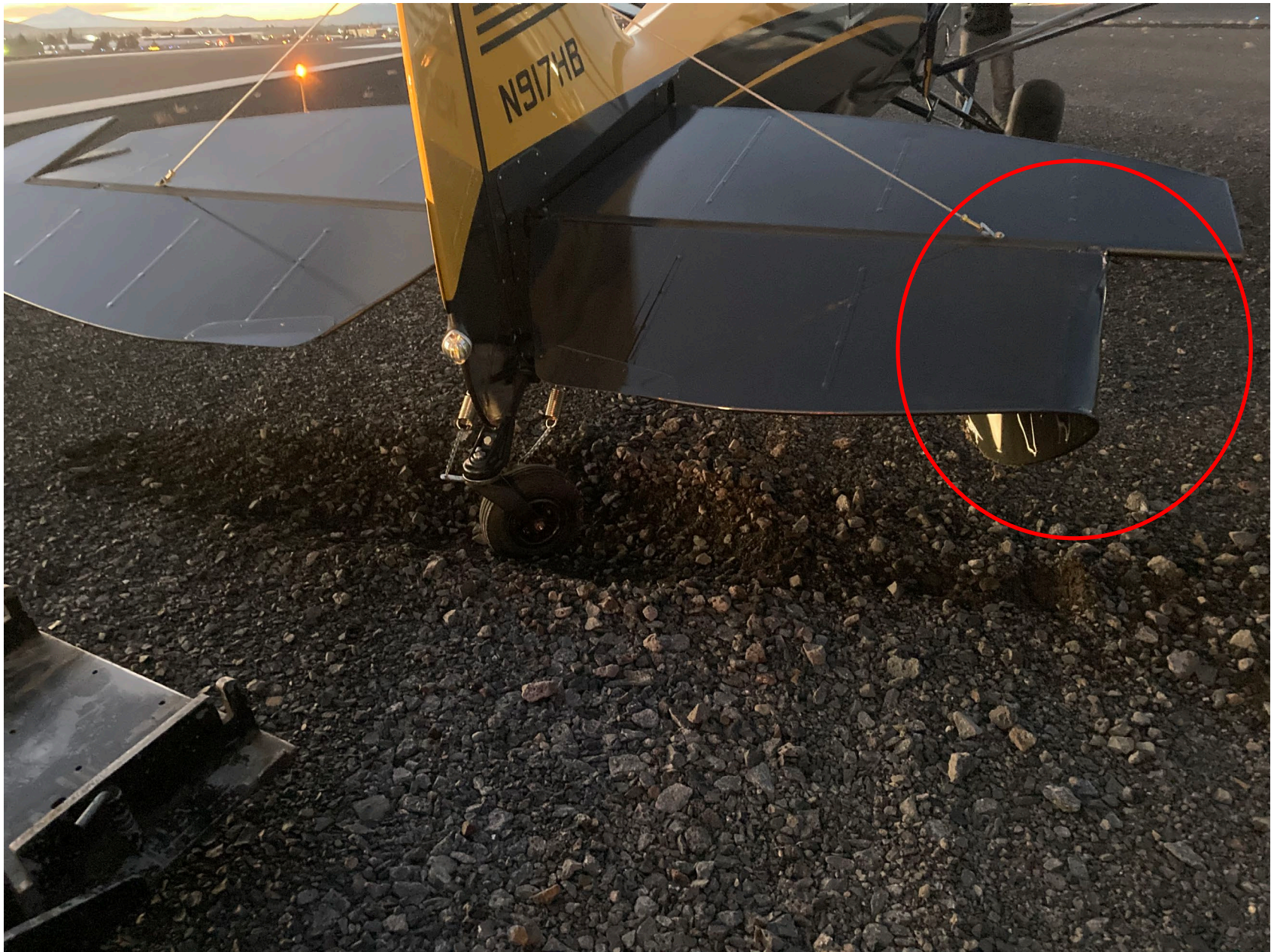
Photo 2 - View of elevator damage (photo courtesy of the pilot)
