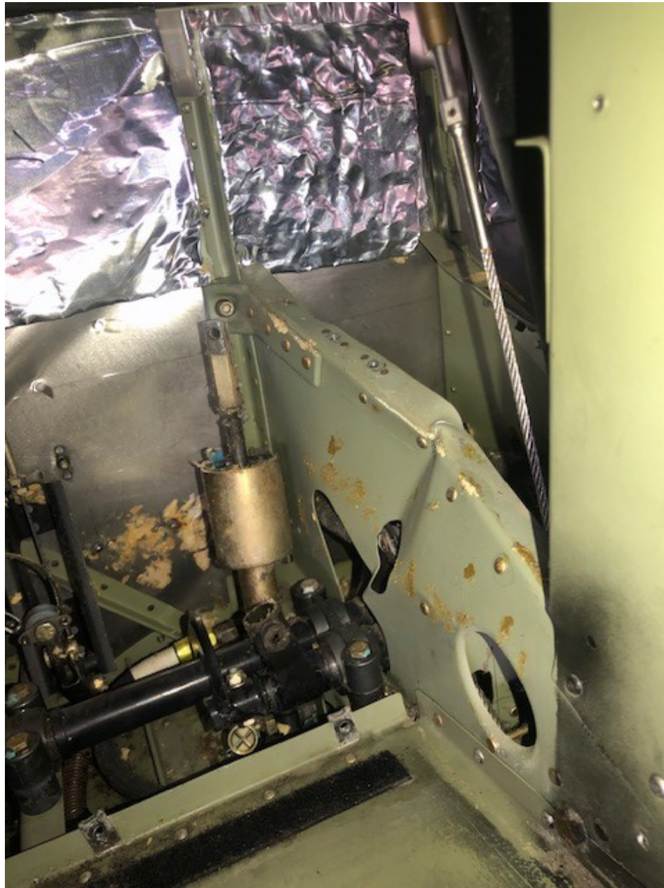
Photo 2 - View of bulkhead assembly damage (photo courtesy of the operator)
