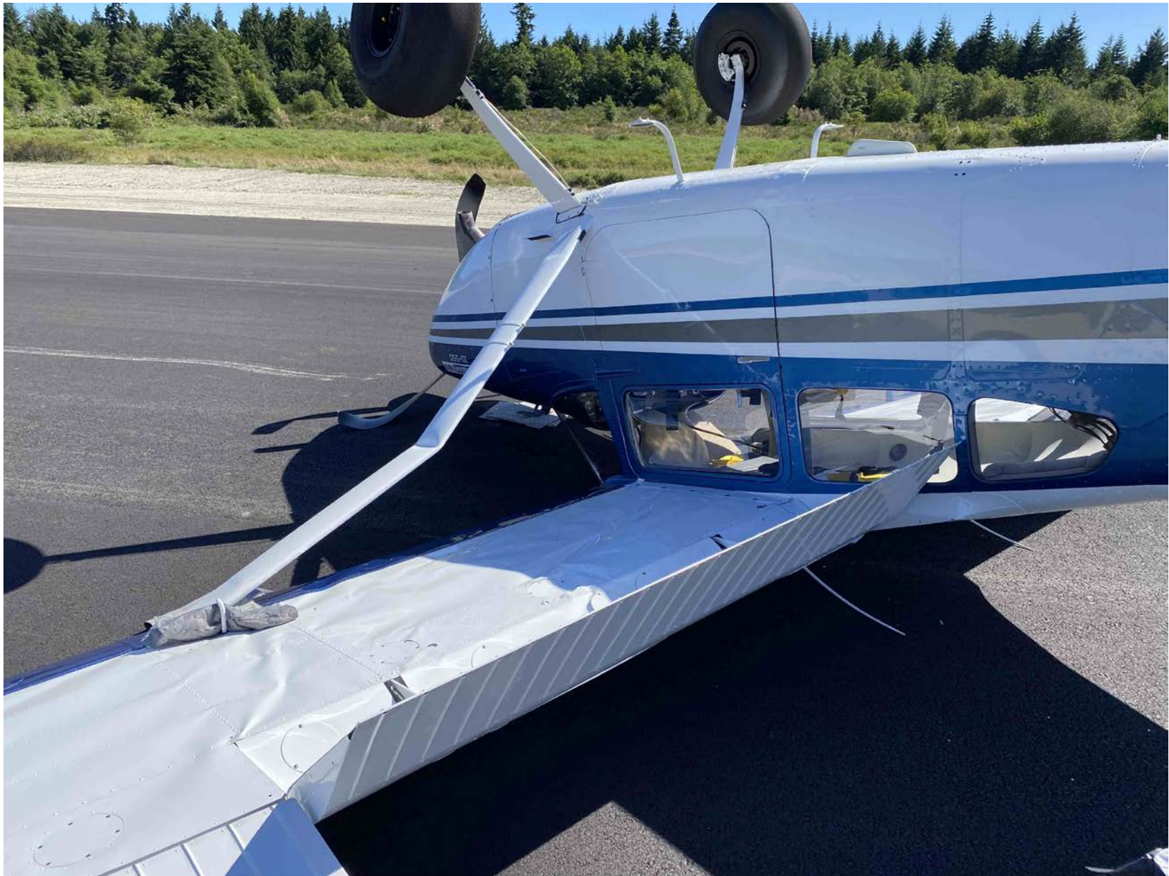
Photo 3 - View of right wing and lift strut damage (photo courtesy of local law enforcement)
