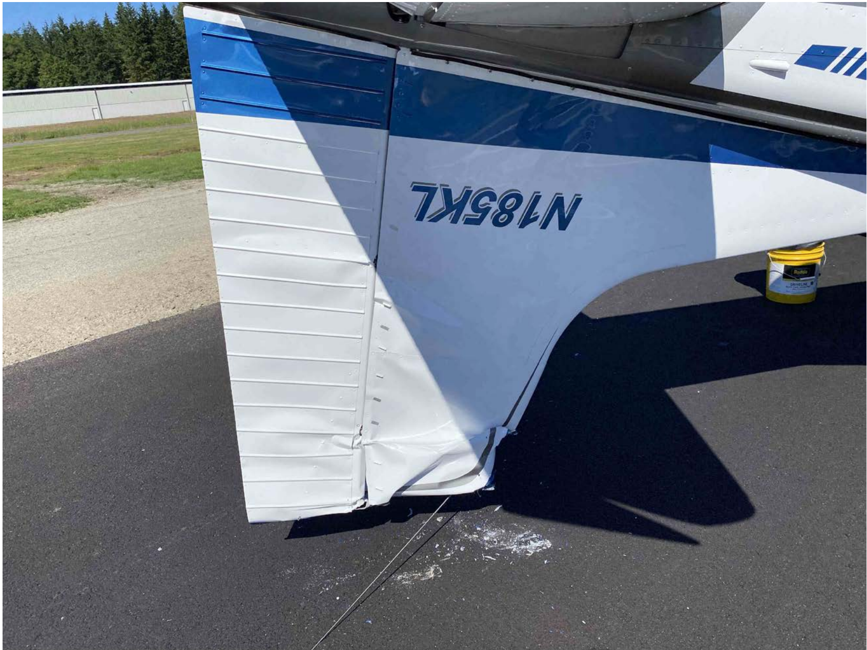
Photo 2 - View of vertical stabilizer and rudder damage (photo courtesy of local law enforcement)
