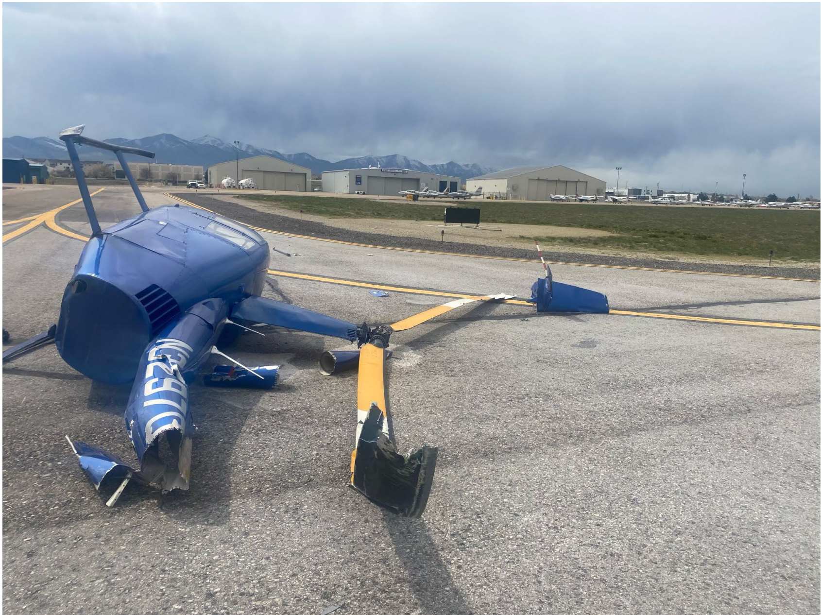
Photo 1 – View of helicopter tailboom damage (photo courtesy of airport operations)
