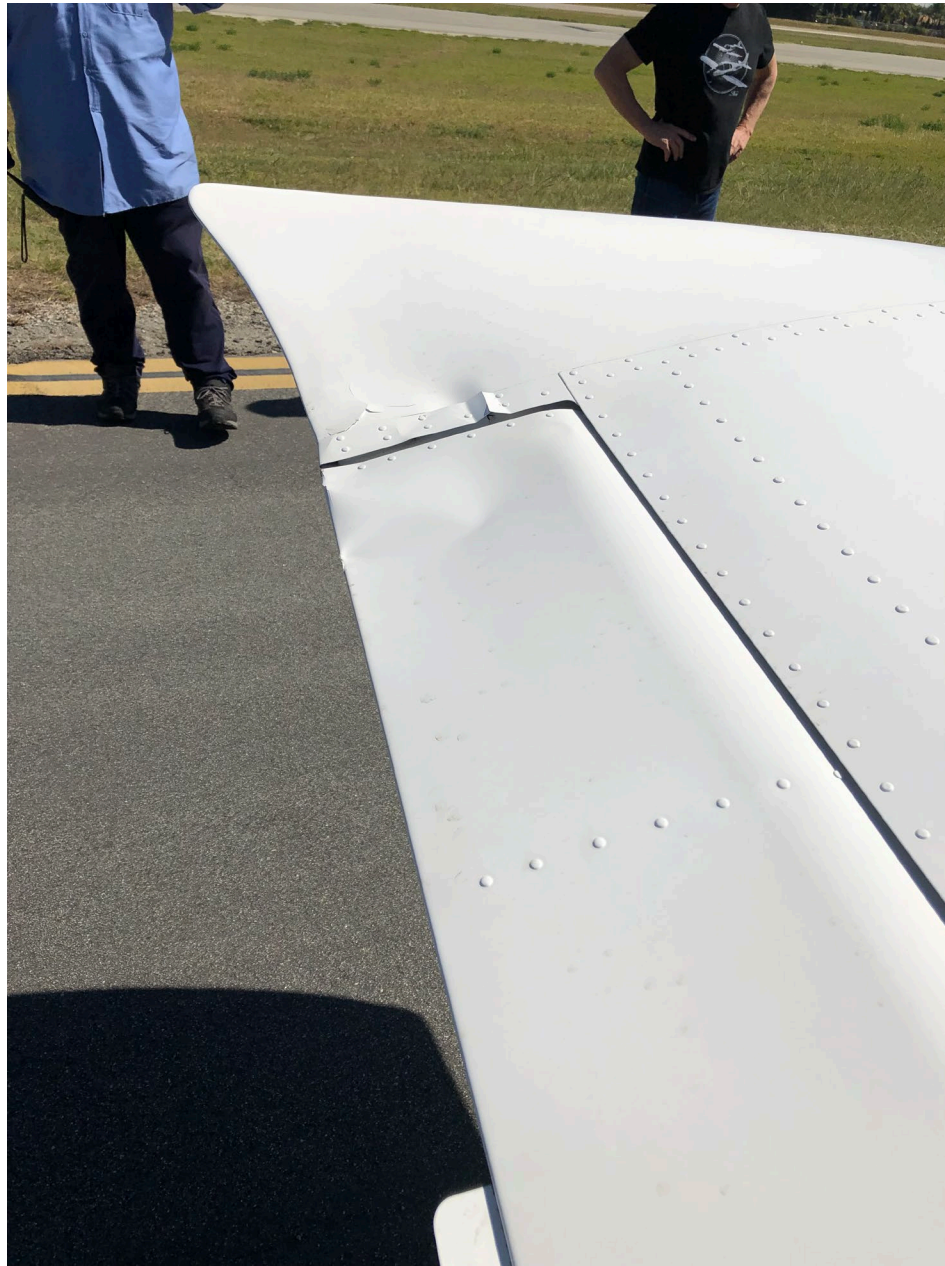
Photo 1 – View of left aileron damage (photo courtesy of the pilot)
