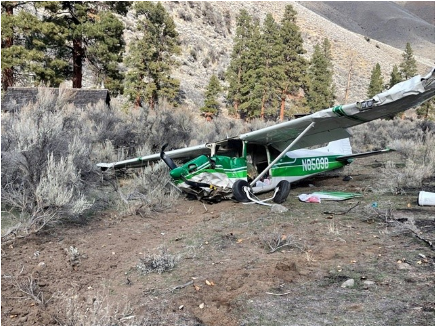
Photo 1 – View of left wing and fuselage damage (photo courtesy of the operator)
