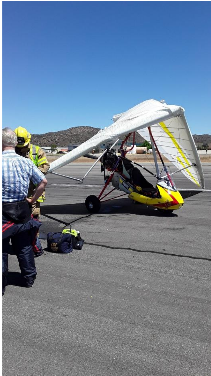
Photo 1 – View of wing damage (photo courtesy of unknown)
