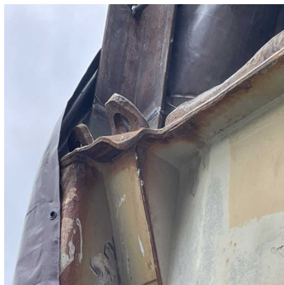
Fixed lashing plate damage on lashing platform fwd. near fr. 86 (3 nos)
