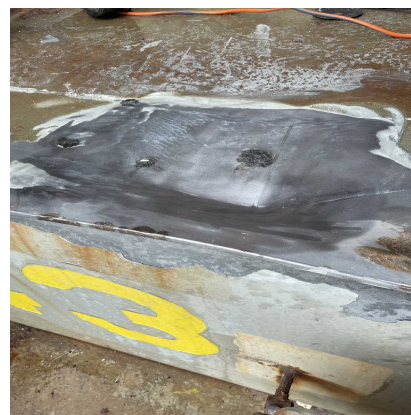
Local deformation on hatch cover 300x300x70mm deep
