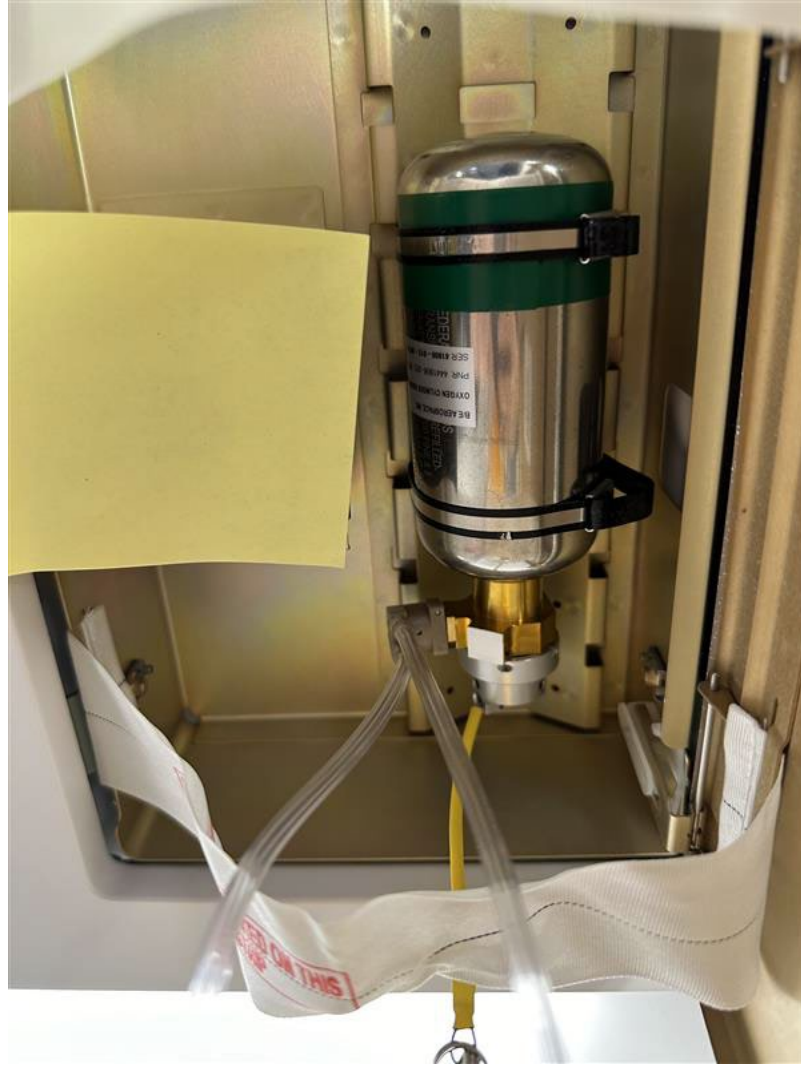
Figure 19. Lav A's CDS oxygen bottle.
