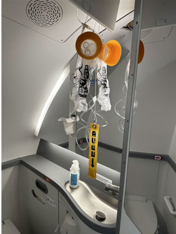
Figure 18. Deployed oxygen masks (with pull tab) in Lav A.
