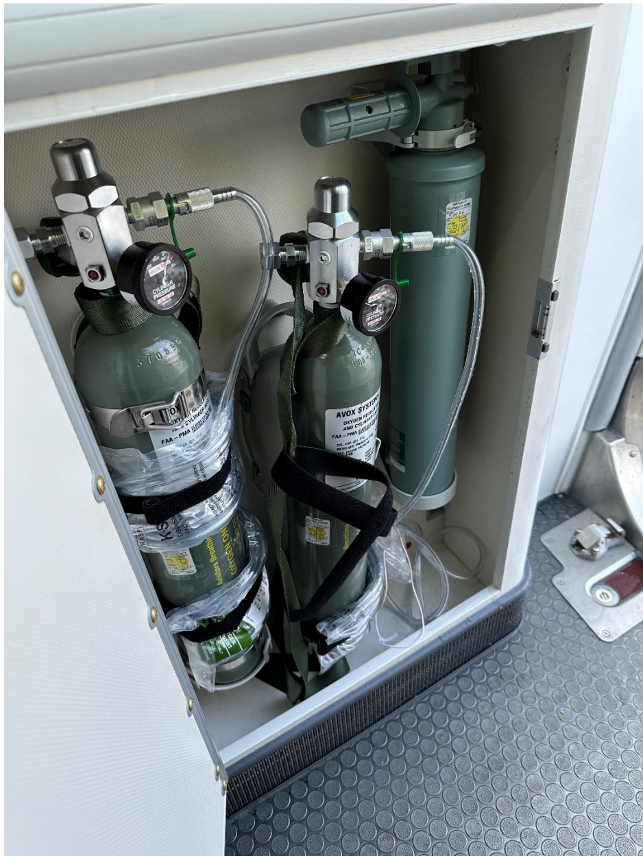
Figure 26. The two POBs in the forward storage location near door L1. The gauge of the unbracketed POB (middle) read 0 psi.
