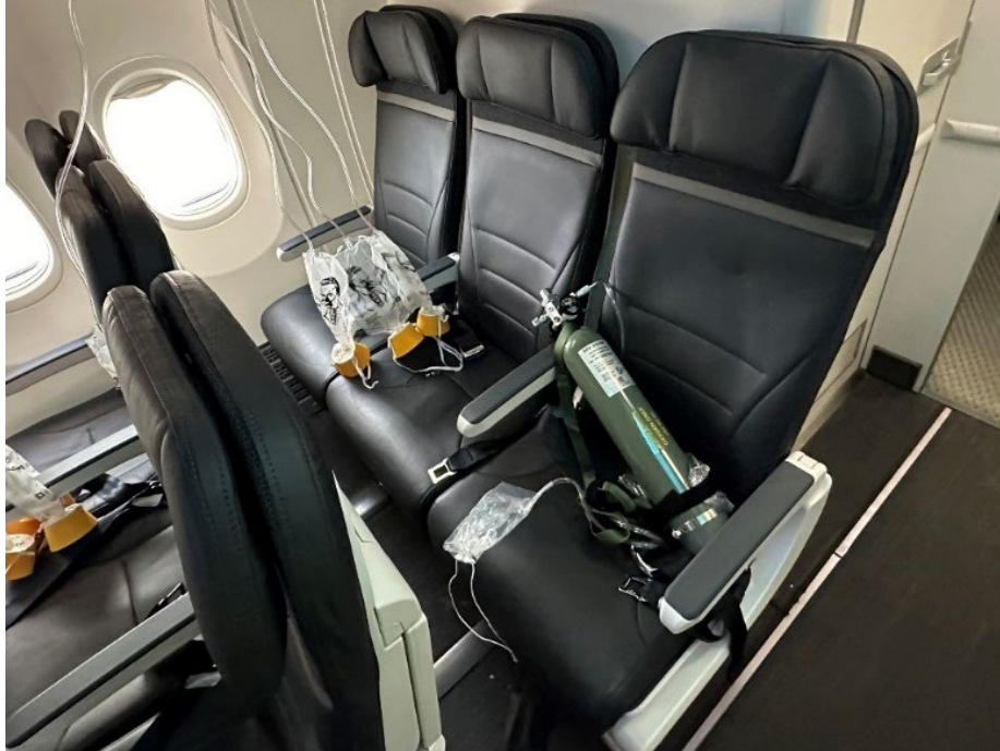
Figure 28. Portable oxygen bottle and mask found on seat 34D.
