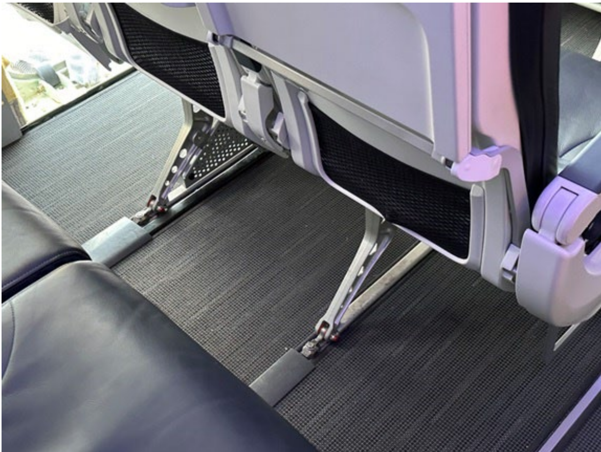
Figure 12. The undamaged aft seat legs of seat unit 26ABC.
