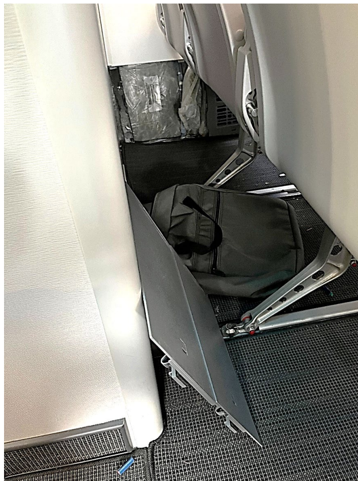
Figure 17. Blank filler panel behind row 32ABC.
