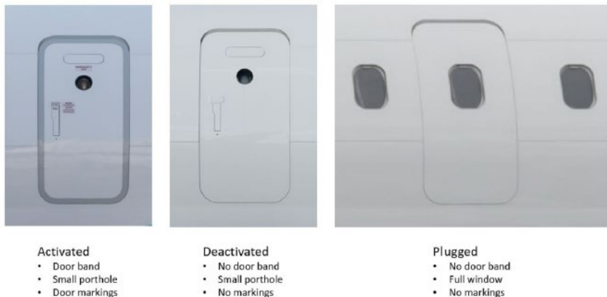
Figure 8. Comparison photograph of the exterior of an airplane fuselage with an activated door (l), a deactivated door (c), and a MED plug (r).
