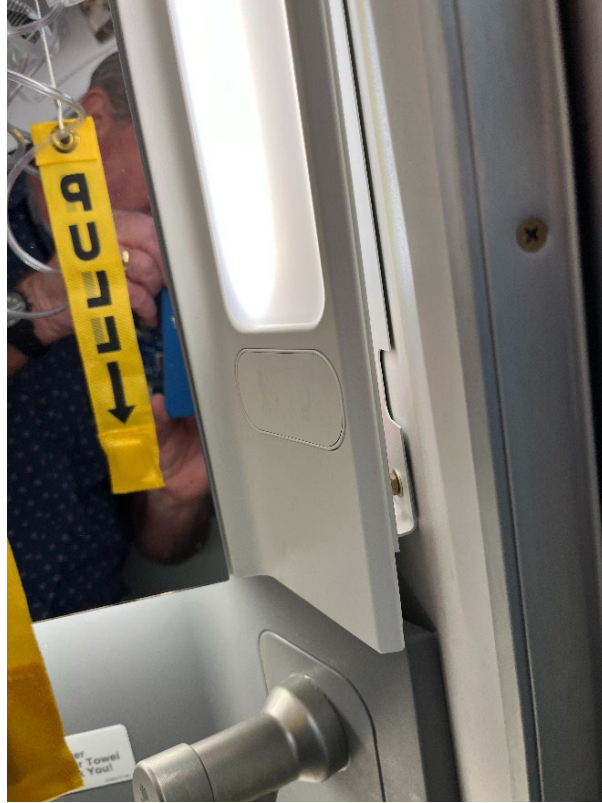
Figure 38. Separation of the Lav A light cover panel from the wall.
