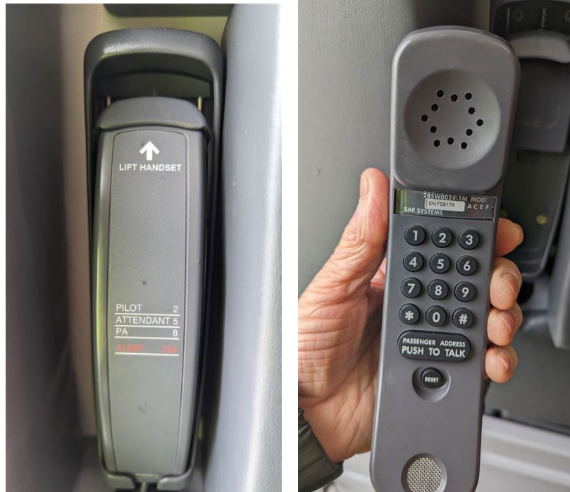
Figure 23. A 737-9 F/A interphone handset.
