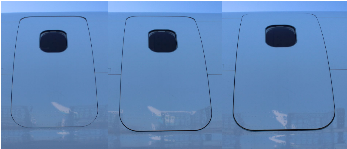
Figure 5. Right MED plug exterior at position A (left), position B (center), and position C (right) [NTSB photos].
