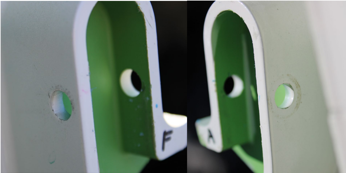
Figure 6. Right MED plug forward (left) and aft (right) upper guide track fitting outboard holes after removal of the upper guide track bolts (NTSB Photos).
