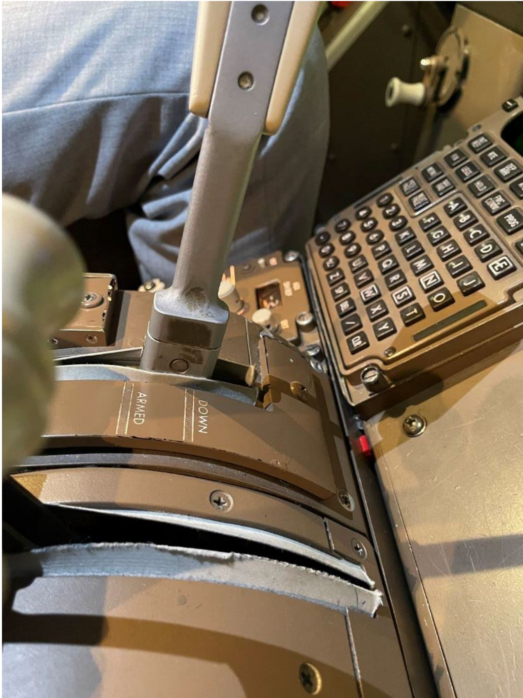
Figure 9: Speed Brake Lever in the "ARMED" Position as viewed from the First Officer's Seat and Lean Forward to look around the thrust reversers. (Source: NTSB)
