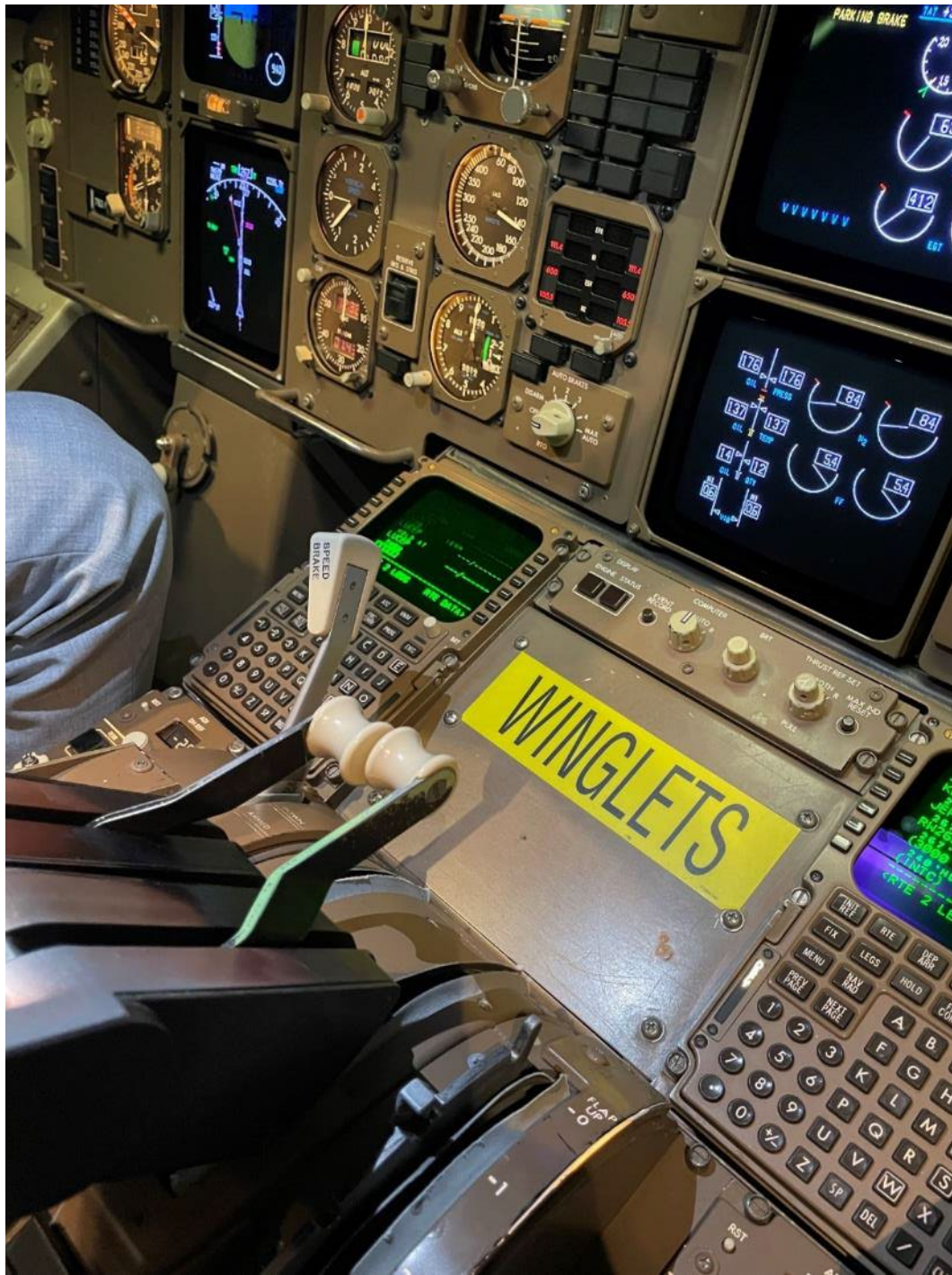
Figure 8: View from First Officer's Seat with Speed Brake Lever in "DOWN" Position. (Source: NTSB)
