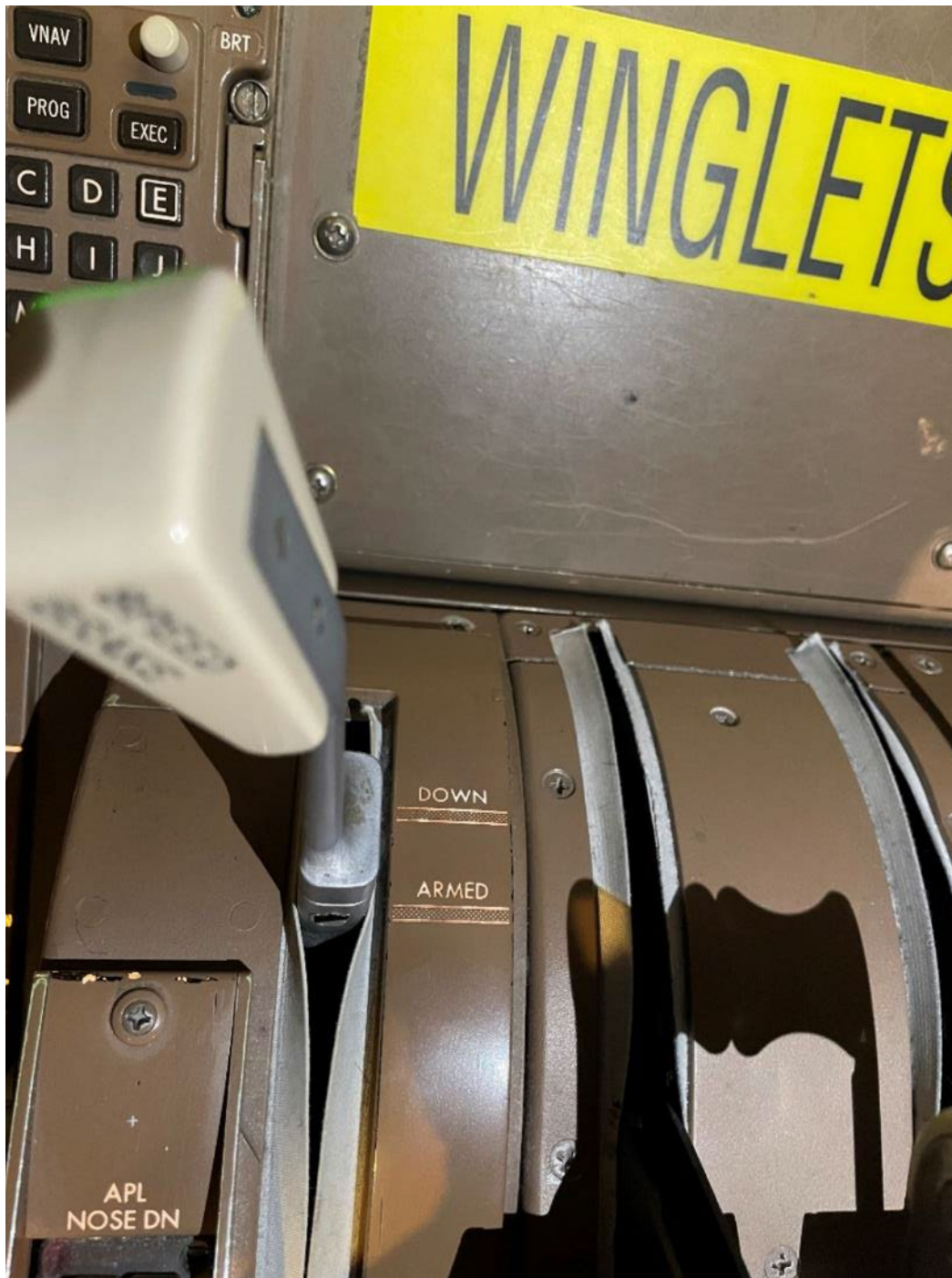
Figure 7: View of Speed Brake Lever in "Armed" Position from Aft of the Center Pedestal. (Source: NTSB)
