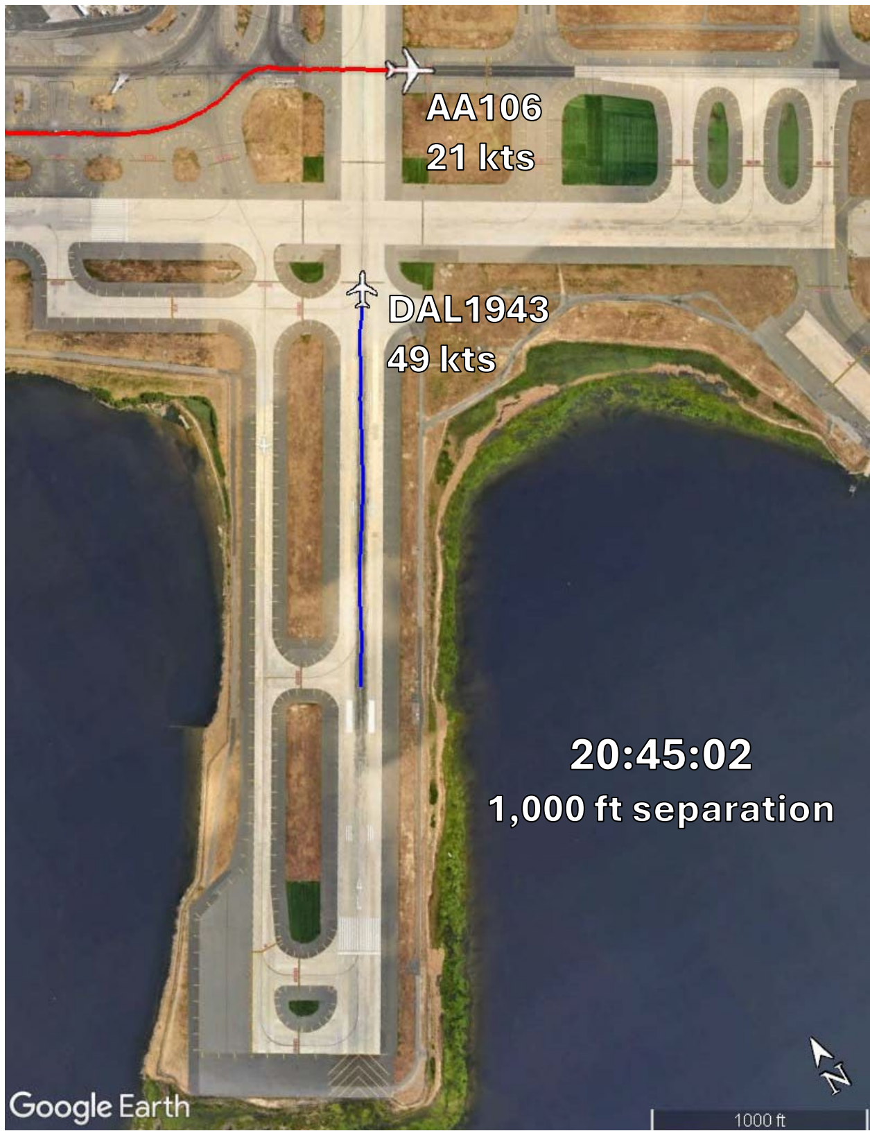
Figure 12. Locations and groundspeeds of both airplanes when AA106 clears runway 4L at 20:45:02.
