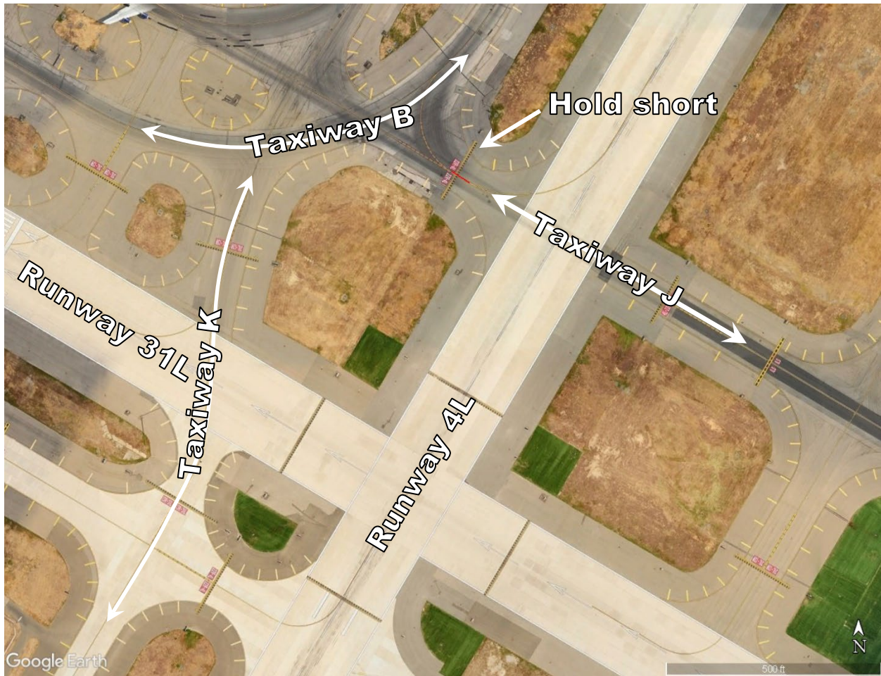
Figure 4. Satellite image of the area of interest. Taxiways B, K, and J and Runways 4L and 31L are labeled as is the hold short line on taxiway J before runway 4L.
