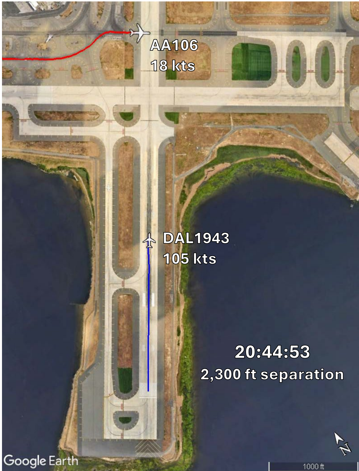
Figure 11. Locations and groundspeeds of both airplanes when DAL1943 was at its maximum speed at 20:44:53.
