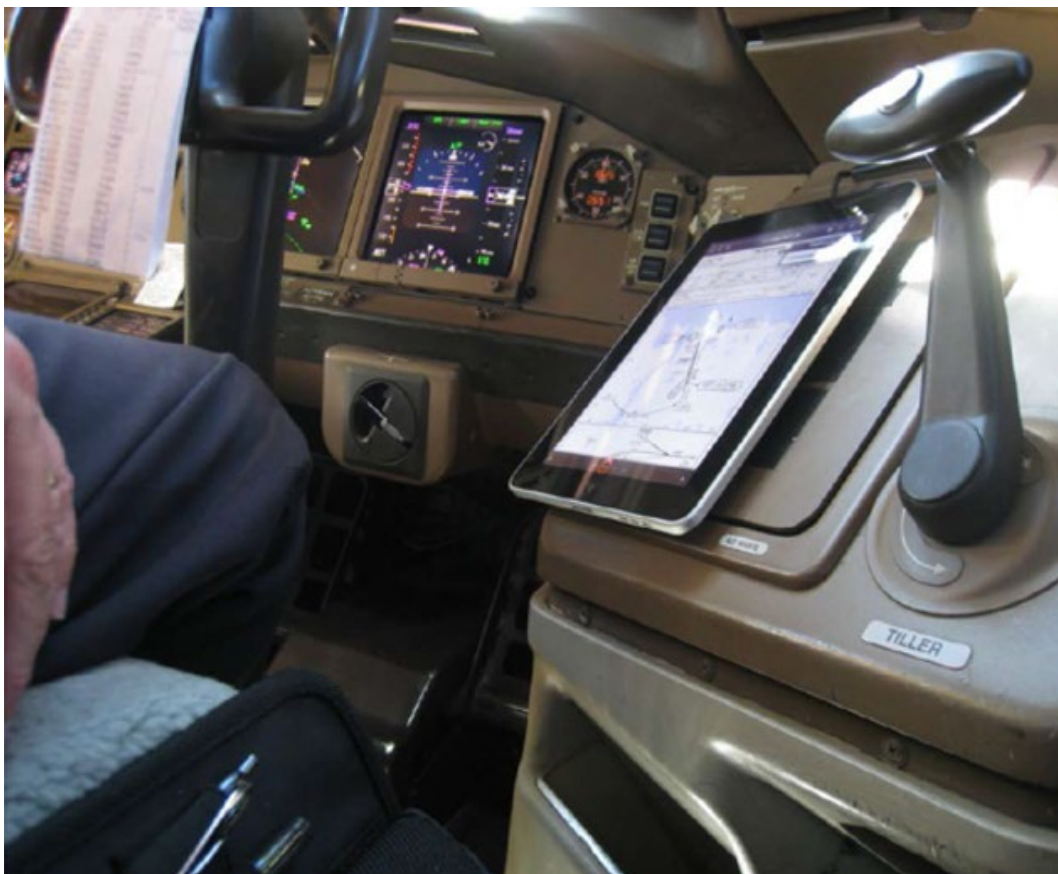
Figure 2. The first officer's iPad mount in the cockpit of an American Airlines B777.
