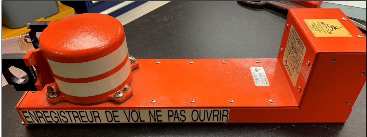
Figure 1. FA2100 from airplane 2 (American), as received.
