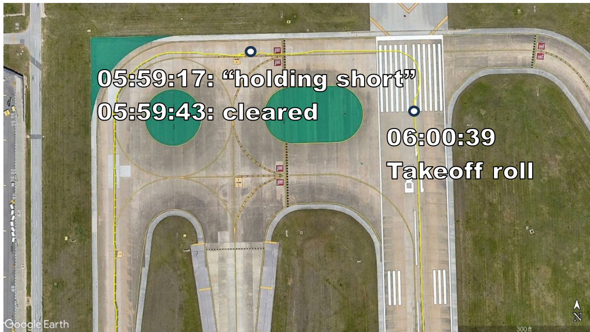
Figure 7. SWA785's departure. Time was 1:22 from clearance to take-off roll.
