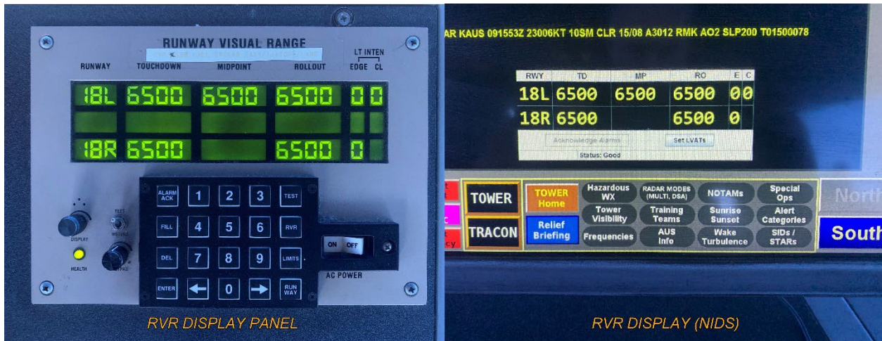
Figure 6. Photographs of RVR Display Panel (left) and the RVR Display on NIDS (right) - (NOT the values from the time of the incident).
