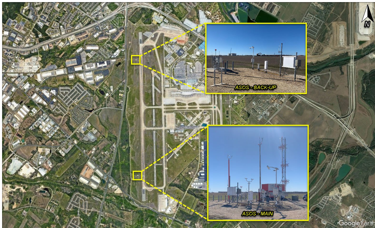
Figure 4. Location of ASOS Main and Backup weather sensor arrays.
