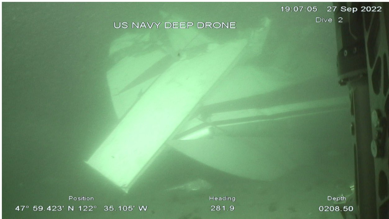
Figure 12. Empennage upright and right side of horizontal stabilizer on seafloor
