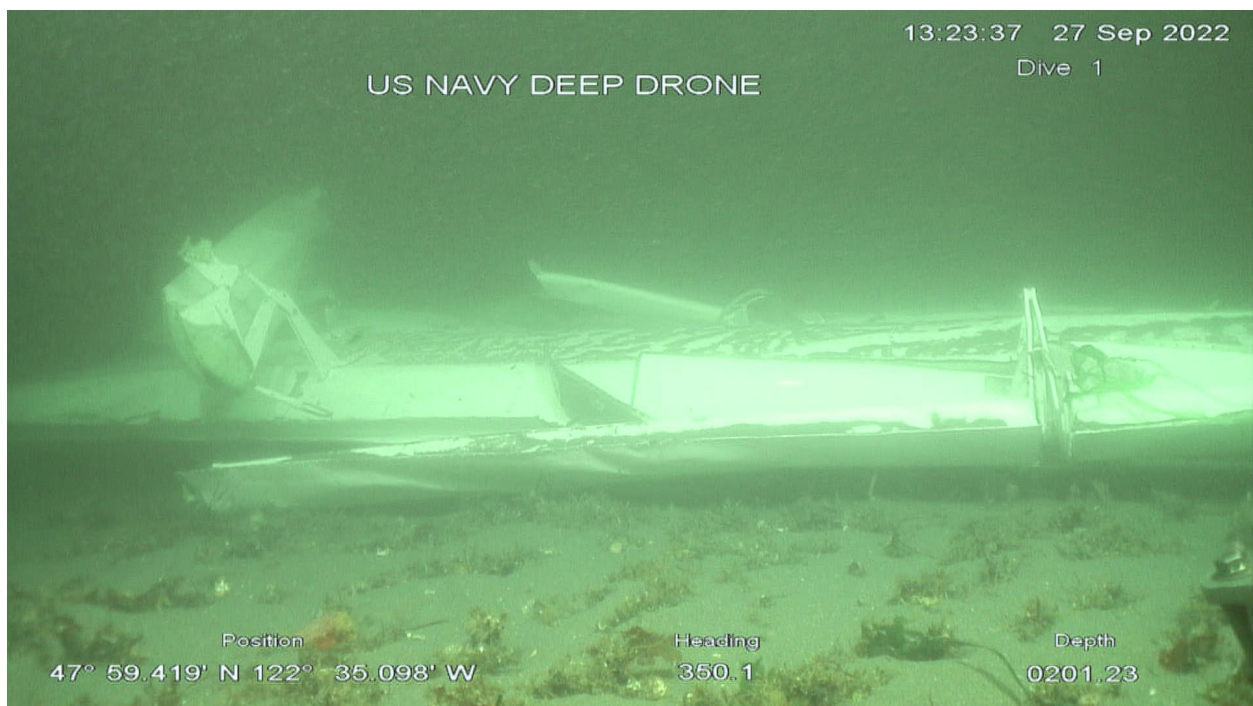
Figure 7. Left wing inboard end on seafloor
