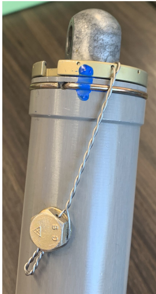
Figure 11. STC modification to horizontal stabilizer actuator clamp nut (NTSB photo)
