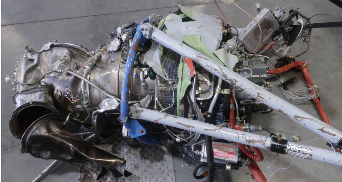
Figure 9. Recovered engine with engine mount attached (NTSB photo)
