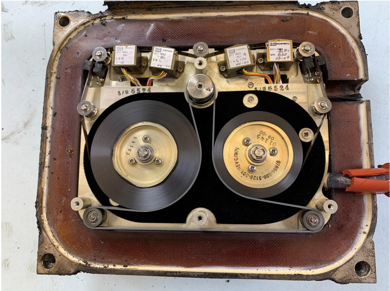
Figure 2. Interior of the Crash Survivable Memory Unit (CSMU) showing the magnetic tape mechanism.
