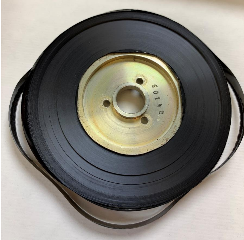
Figure 3. Magnetic tape removed from recording mechanism showing deformed tape wrapped around the center spool.
