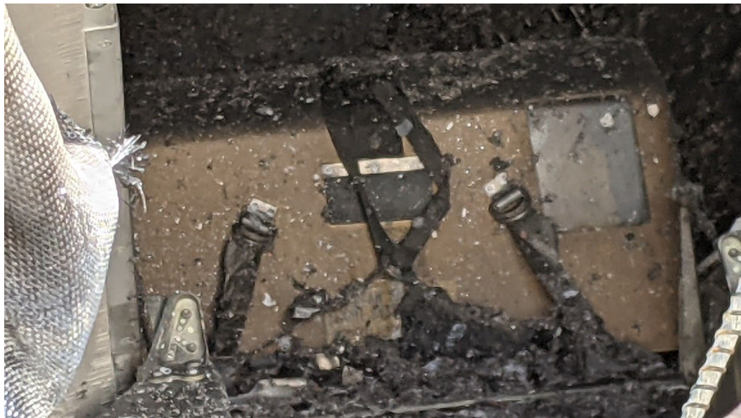
Photograph 9. N987AK tailcone slide still in packaging.
