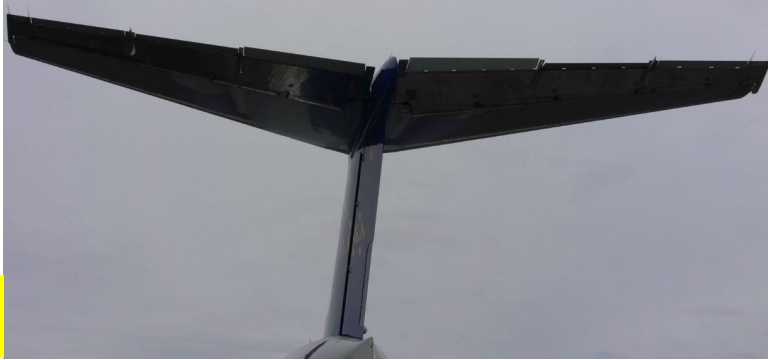
Figure 7: Elevator and Rudder Preflight Inspection. (Source: Everts Air Cargo Training Walkaround)
