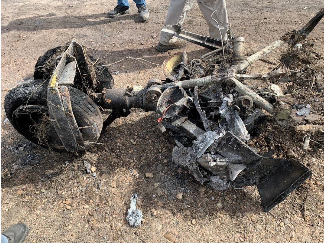
Figure 16. The nose landing gear after removal from underneath the airplane fuselage.
