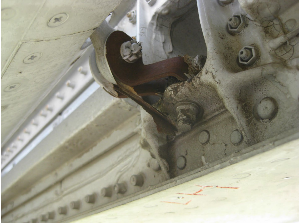
Figure 26. Left-hand elevator inboard geared tab attachment linkage, looking forward (into the horizontal stabilizer) and outboard, viewed from underneath the left elevator.
