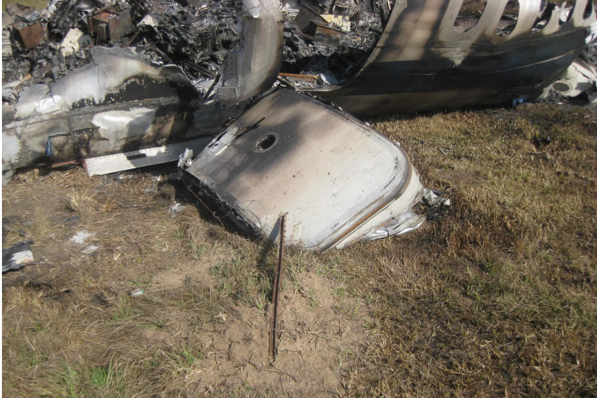
Figure 14. The forward left entry door, with fuselage wreckage.
