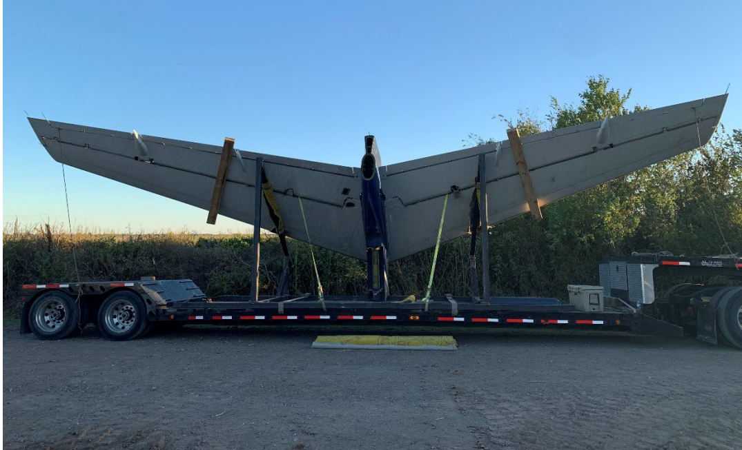
Figure 30. The airplane's tail structure placed onto trailer prior to movement to the wreckage storage facility.
