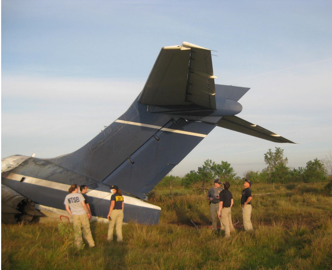
Figure 21. The left side of the vertical stabilizer and rudder. Note that the elevators are in a trailing edge down position.
