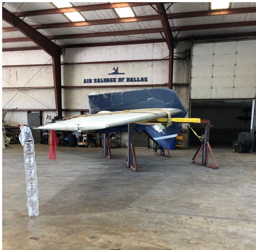
Figure 33. Airplane's tail section prior to disassembly and examination by the group.
