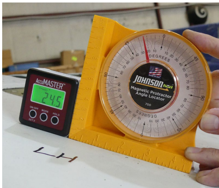
Figure 34. Digital calibrated inclinometer showing elevator throw movement measurement.
