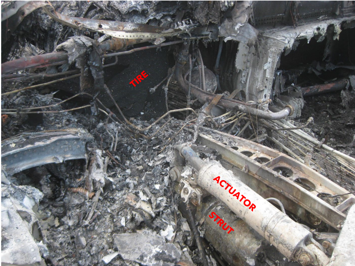
Figure 18. The right main landing gear, as found in the main wreckage. The gear strut, strut actuator, and one of the tires have been annotated.
