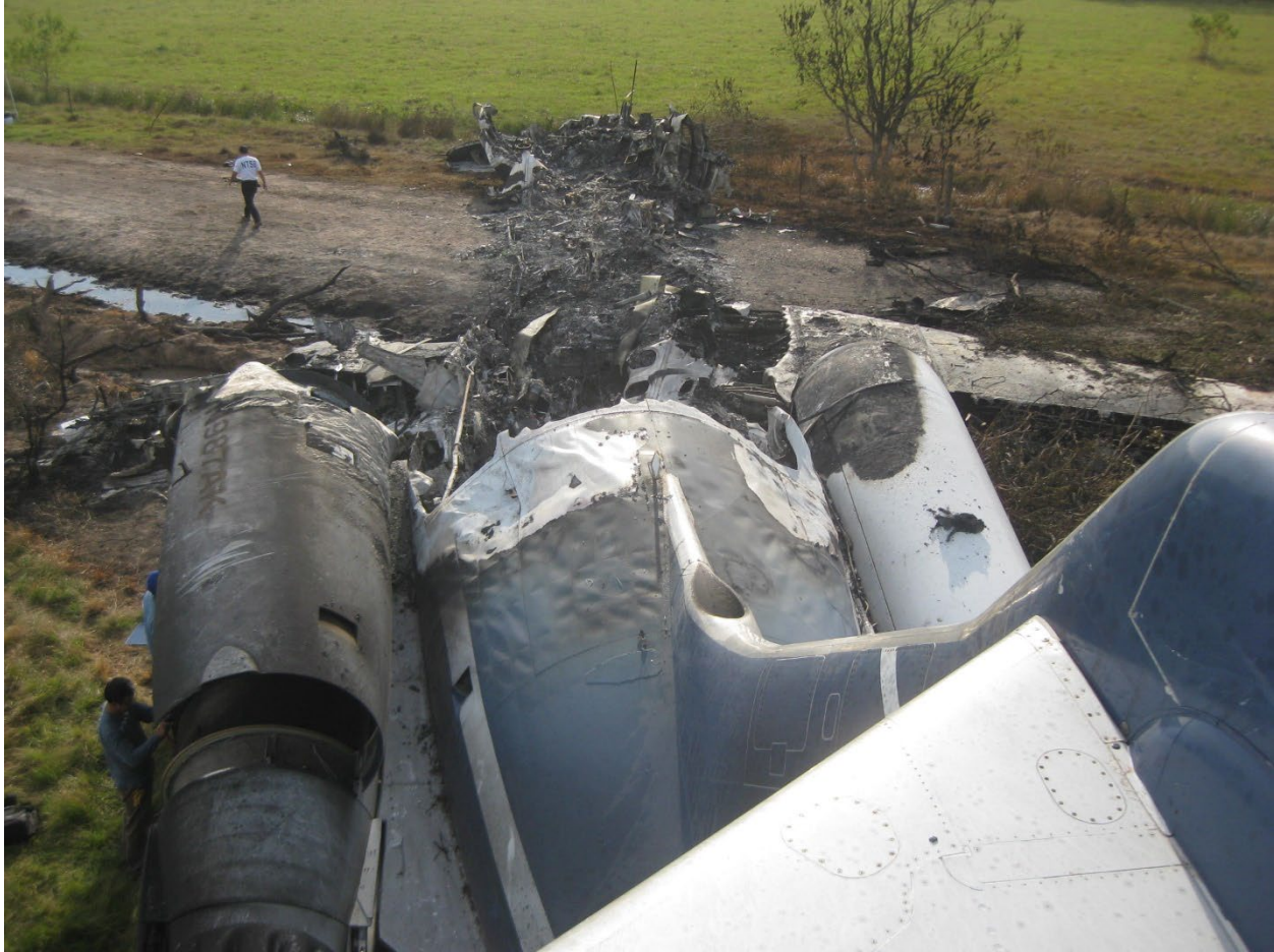
Figure 9. Photograph from top of the horizontal stabilizer, looking forward, of the forward fuselage and damage from post-crash fire.
