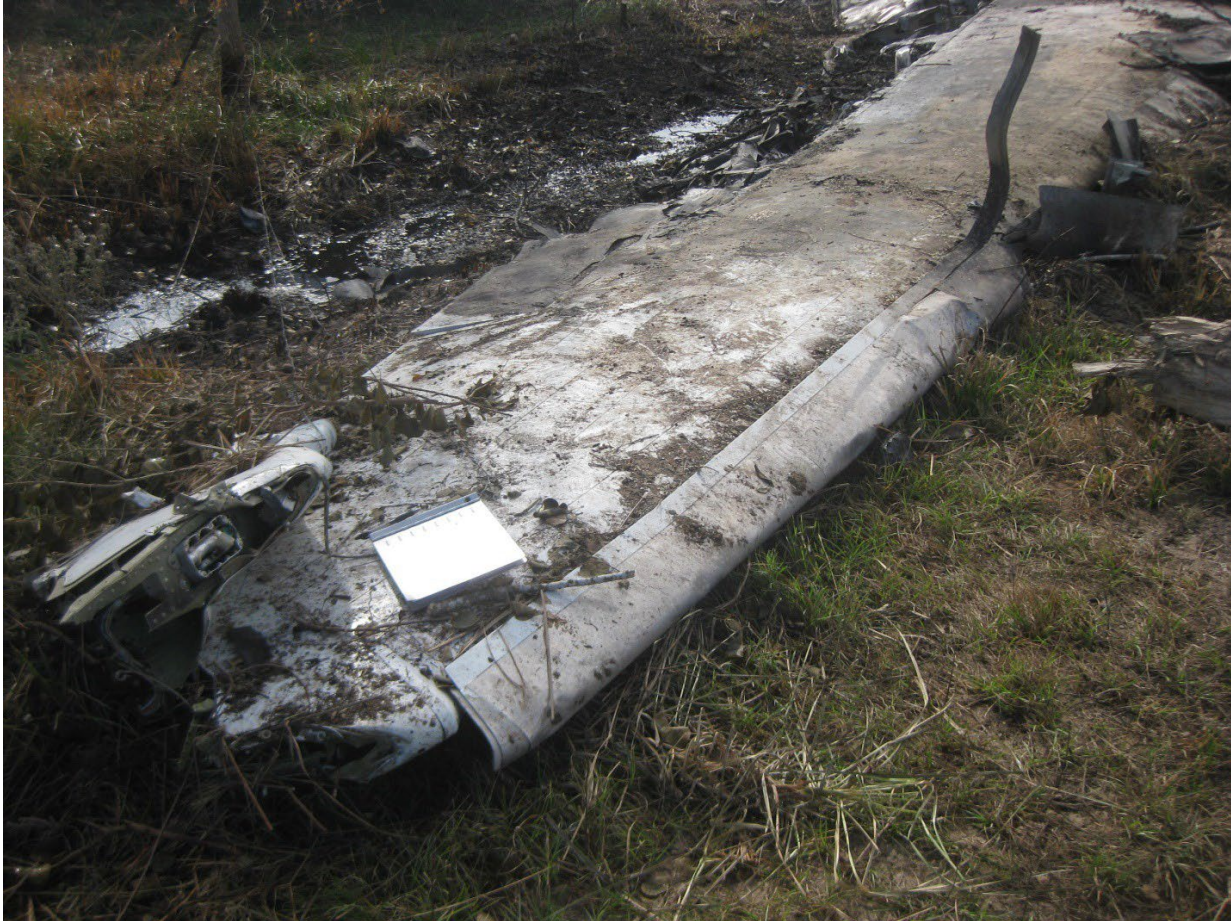
Figure 11. View of right wing after debris was removed from top of the wing, looking from wingtip inboard.
