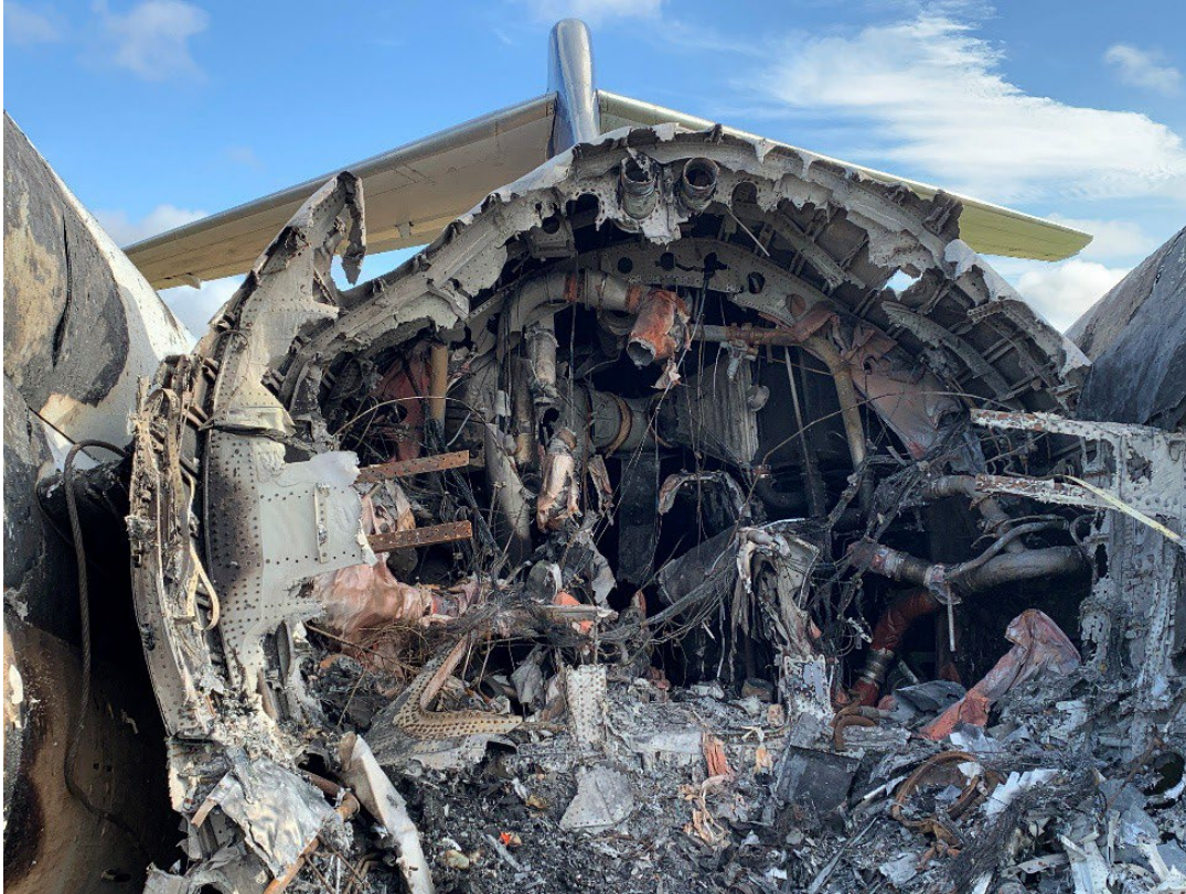
Figure 19. Area of the aft pressure bulkhead, showing the area consumed by post-crash fire.
