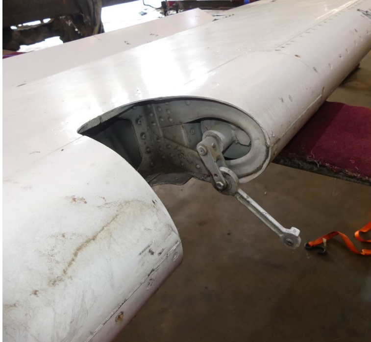
Figure 35. The left elevator damper, as installed, with linkage extended.
