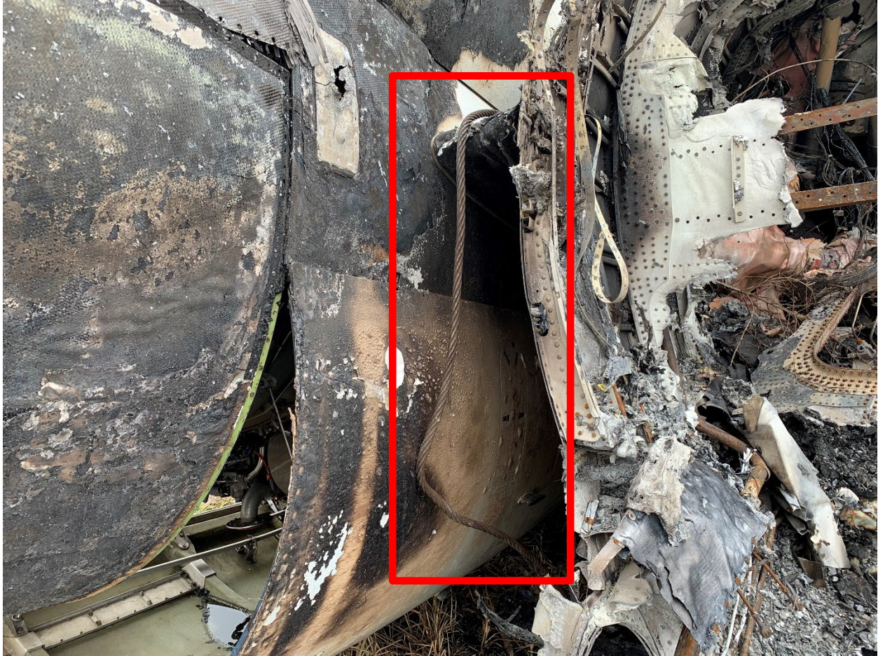
Figure 3. Piece of electrical distribution line, highlighted in red box, found on Number 1 Engine pylon.
