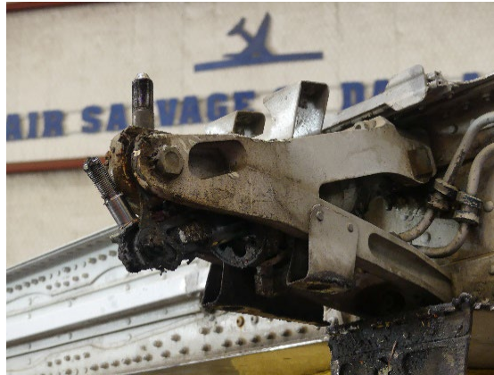
Figure 37. The left-hand hydraulic boost cylinder, as installed.
