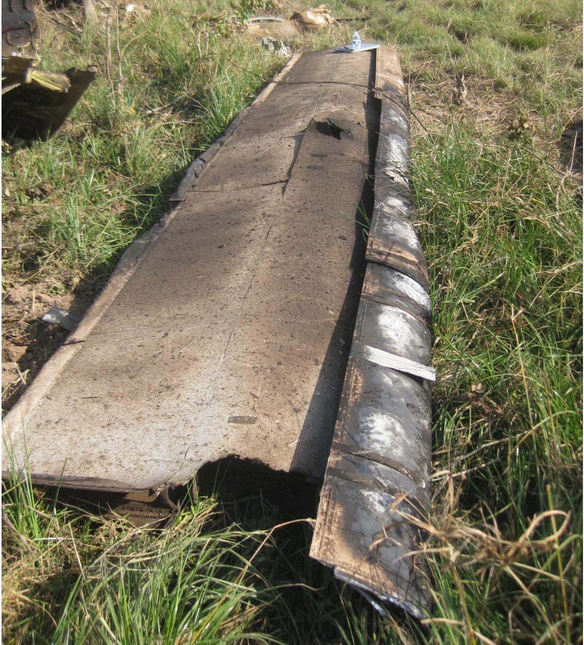
Figure 12. A section of the outboard left wing, located in the wreckage path. The wing's leading edge is on the right side of the photograph.
