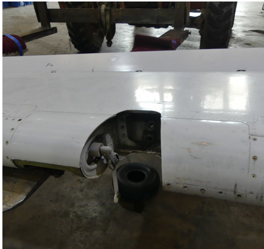
Figure 36. The right elevator damper, as installed, with linkage extended.
