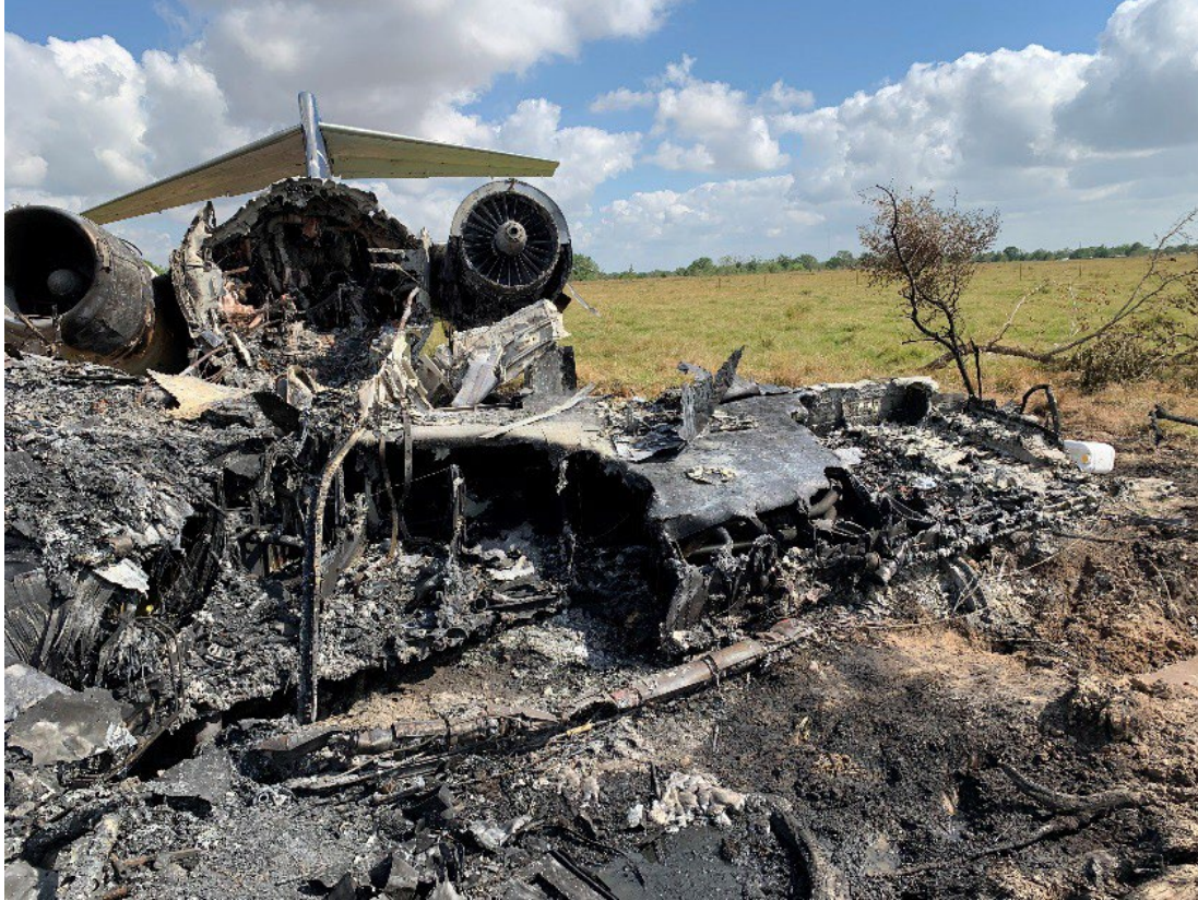
Figure 13. Section of left wing, still attached to the fuselage.
