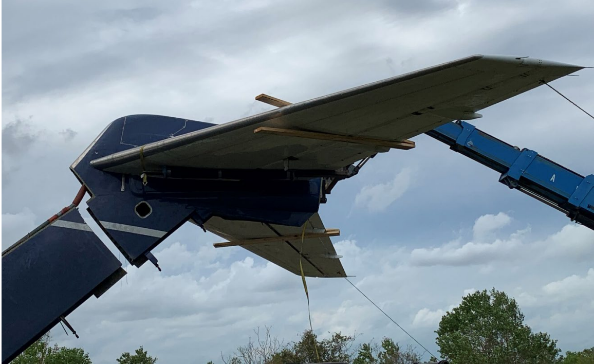
Figure 29. Cutting of the vertical stabilizer after the rudder and stabilizer spar cap were removed. Note the wood planks clamped to secure the elevators.
