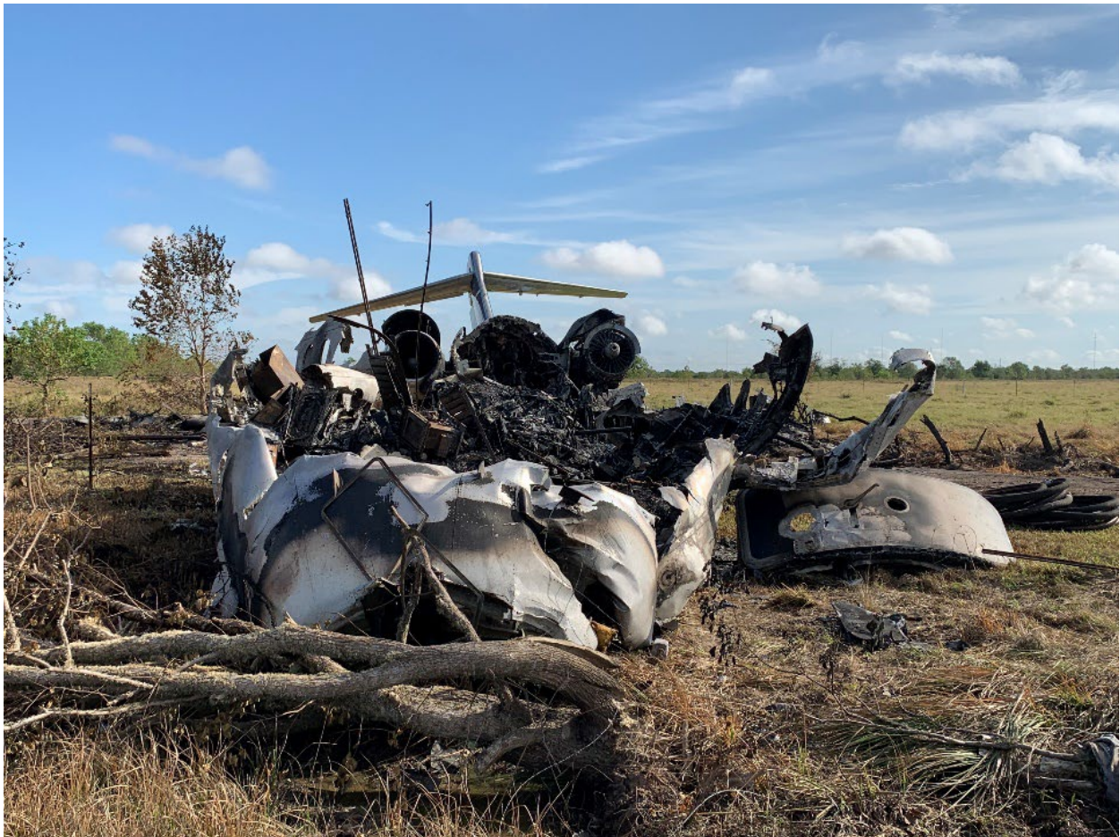
Figure 1. View of airplane fuselage wreckage, from the airplane nose and looking aft.
