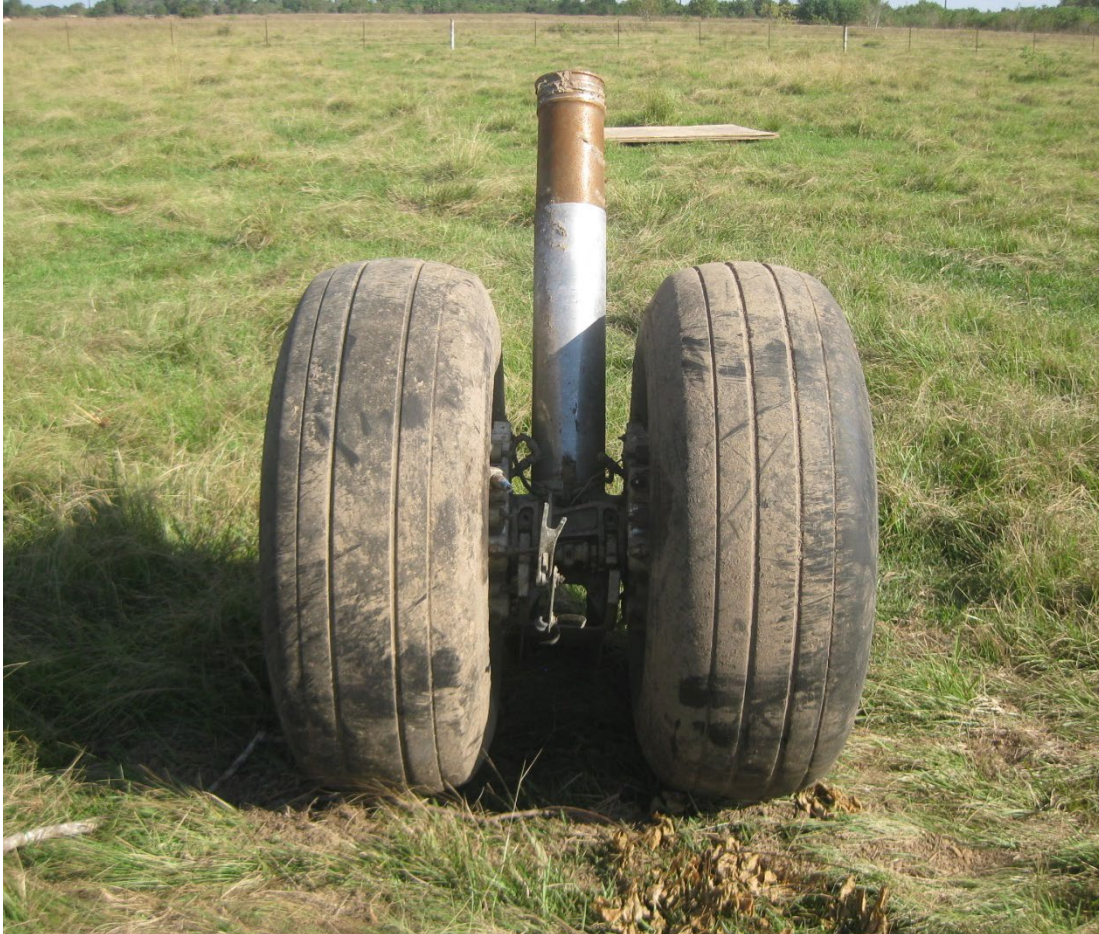
Figure 17. Lower section of left main landing gear, as found in wreckage path.
