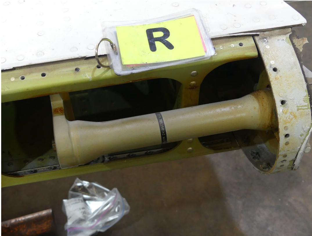
Figure 42. The right elevator torsion bar, as installed.
