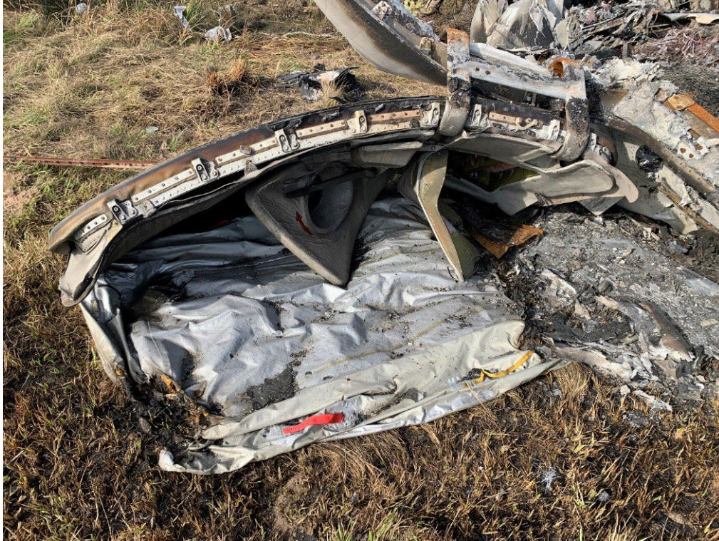
Figure 15. Front left entry door and evacuation slide, looking forward.
