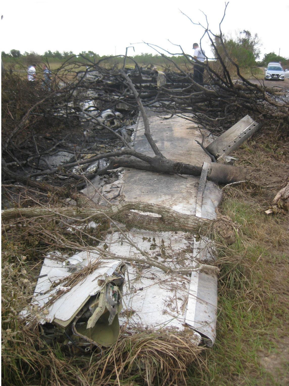
Figure 7. View of right wing, looking inboard from the right wingtip. The wing's leading edge is on the right side of the picture.
