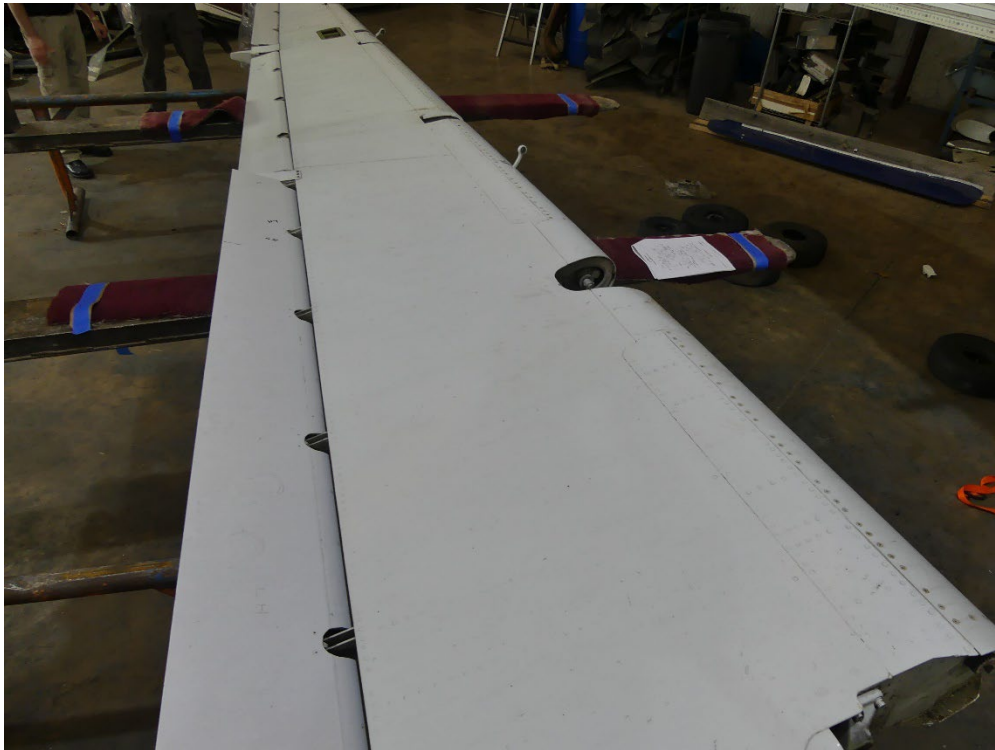
Figure 39. The left elevator control surface after removal, looking outboard.
