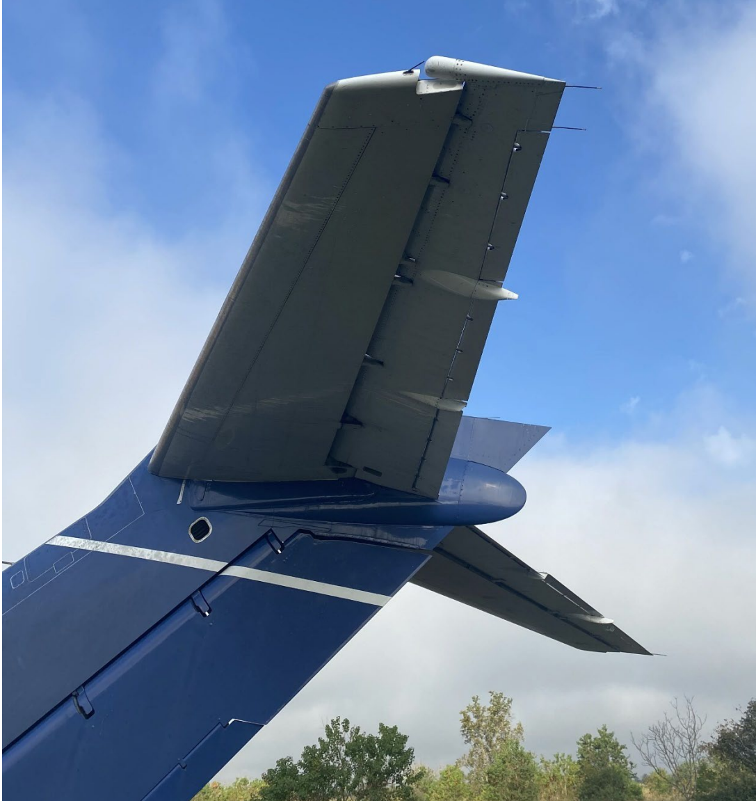
Figure 24. Elevators in the as-found trailing edge down position.
