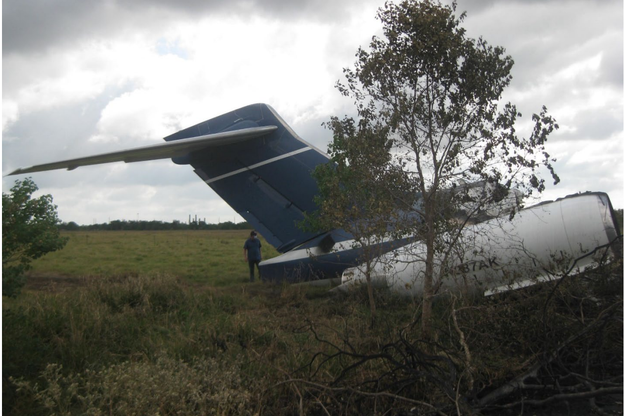
Figure 20. Right side of the vertical stabilizer, rudder, and engine number two.
