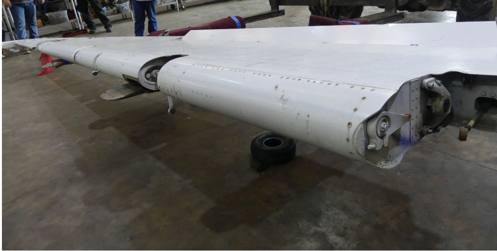
Figure 40. The right elevator, inboard leading edge, looking outboard.
