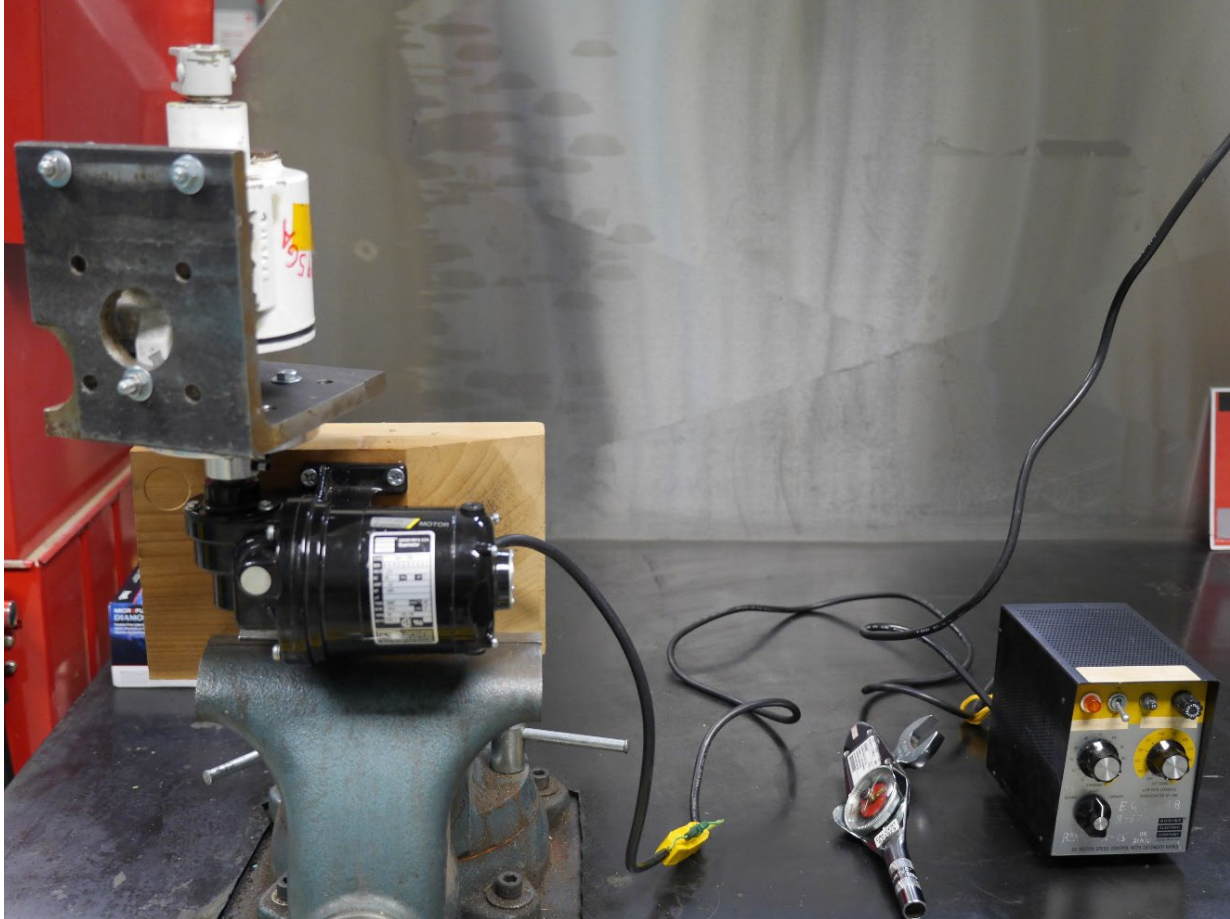
Figure 1. The Elevator Damper Test Rig, with exemplar damper attached.
