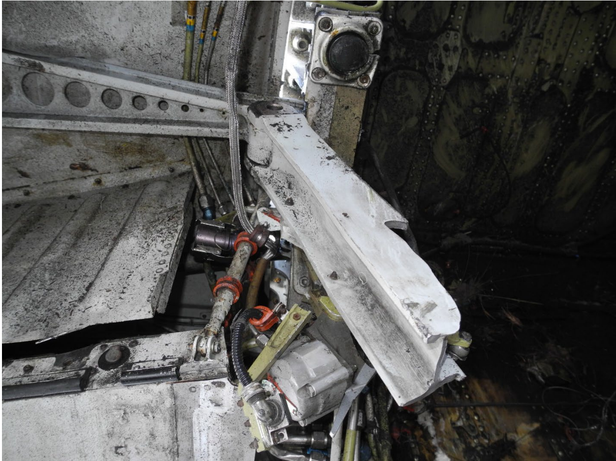
Figure 13 Upper portion of upper side brace
