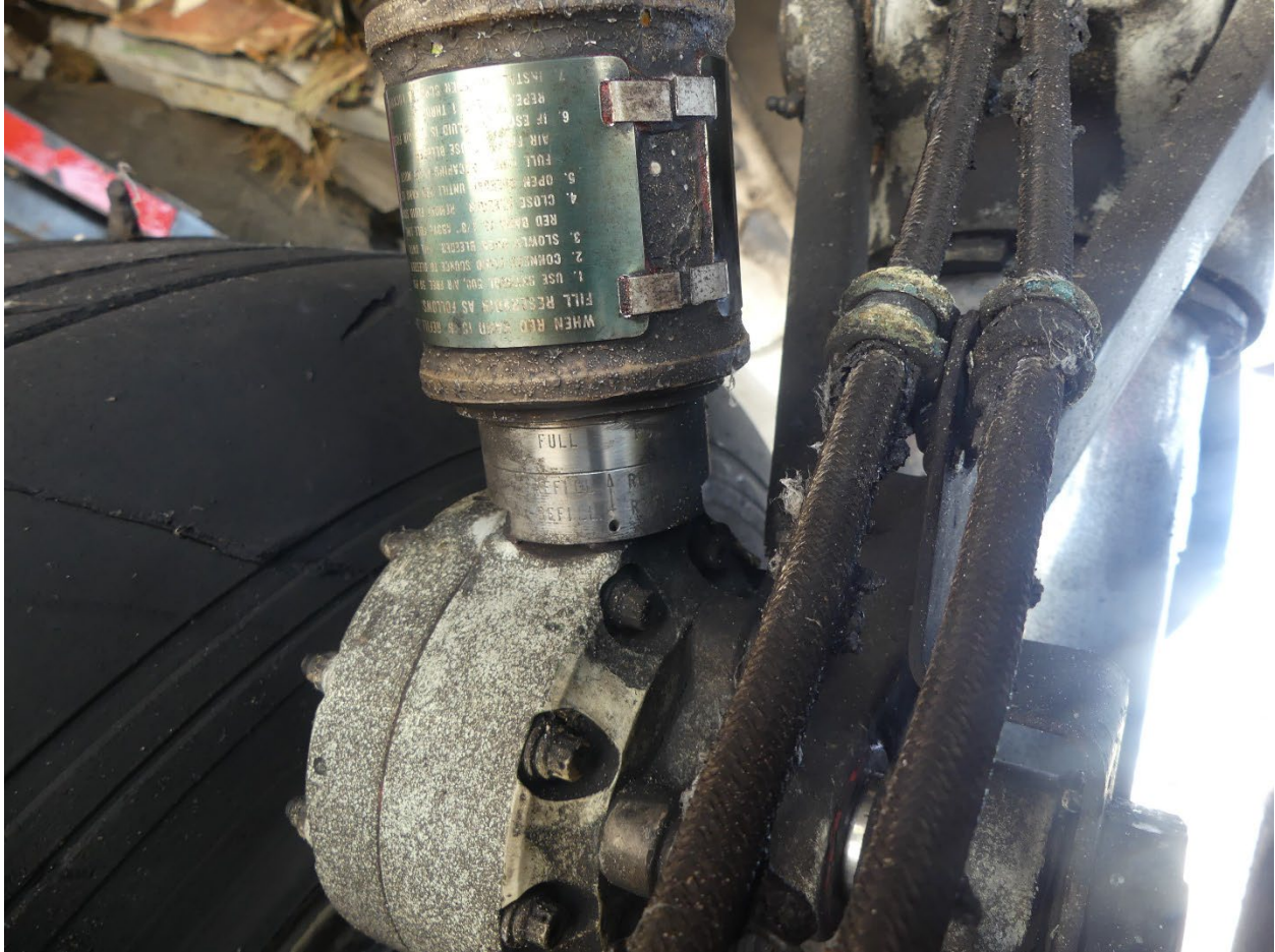
Figure 23 Right gear shimmy damper with hydraulic reservoir intact
