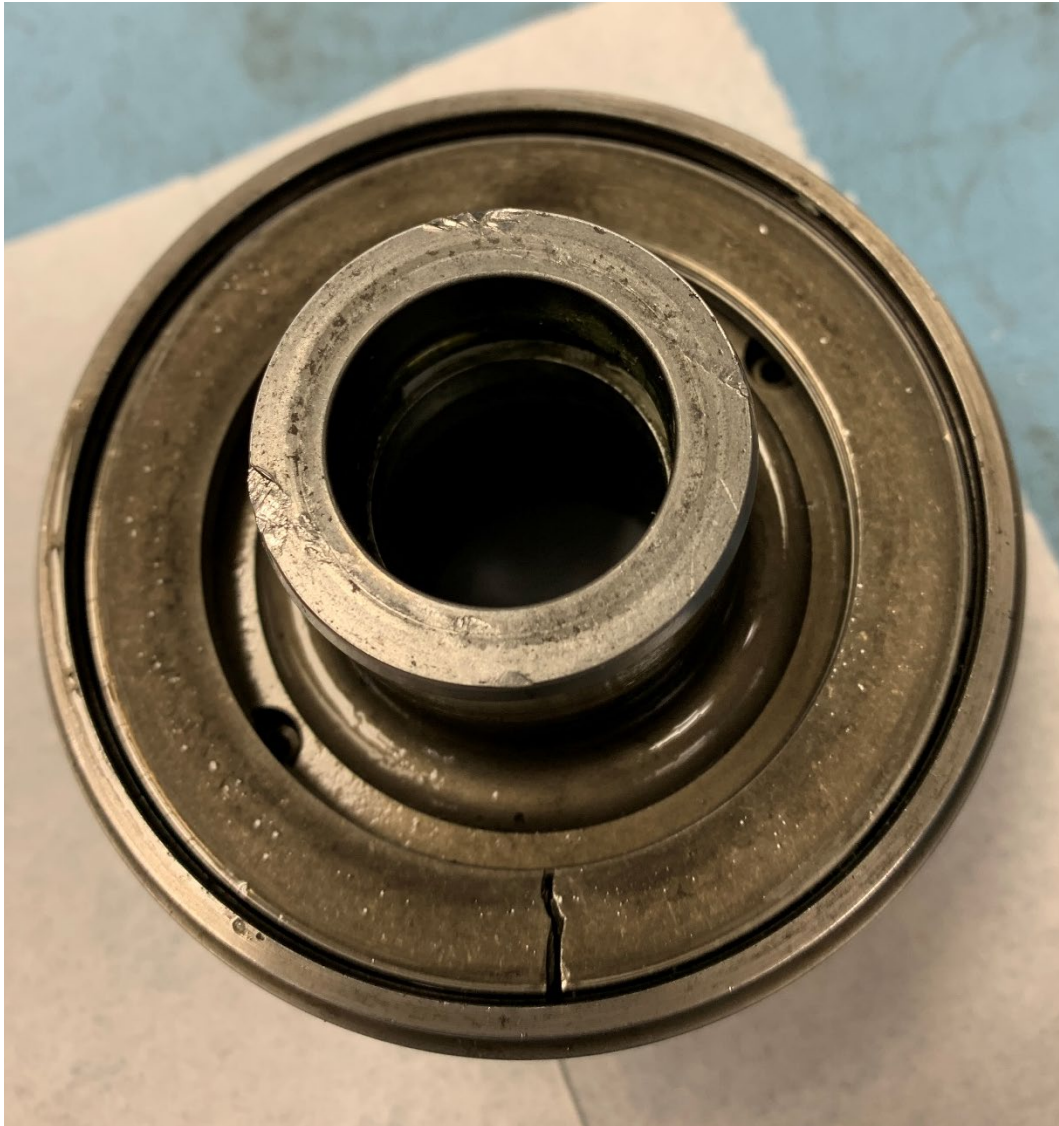
Figure 21 Shimmy damper piston and fractured Belleville washer
