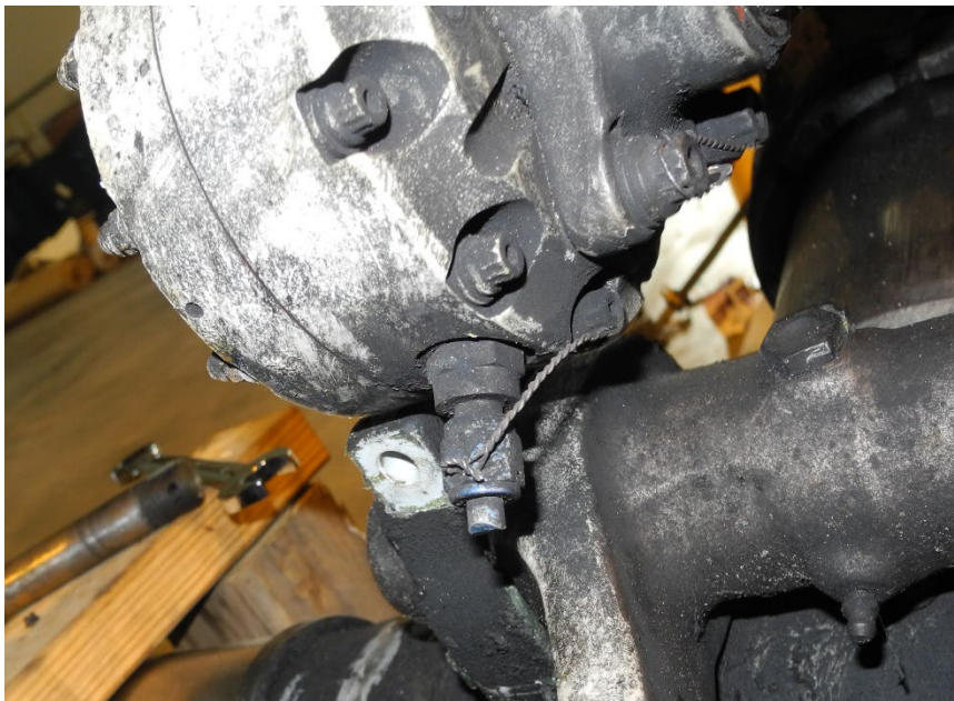
Figure 24 Right gear shimmy damper service port
