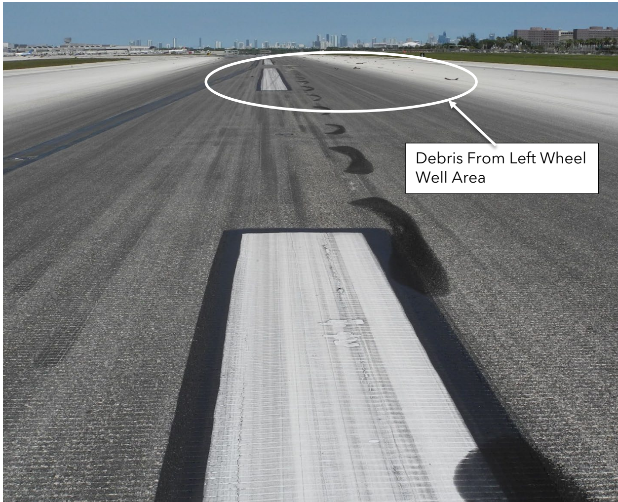
Figure 8 Tire marks after gear collapse
