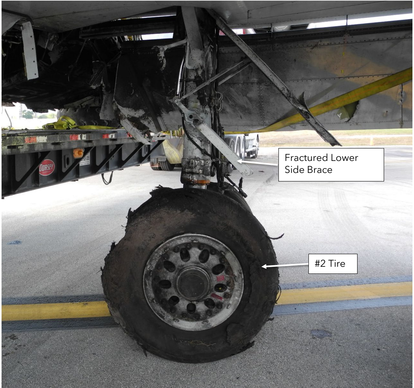
Figure 11 Left main landing gear (looking aft)
